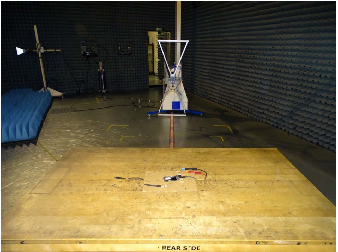
Photo 3: Test setup for radiated measurements in semi-anechoic chamber, 30 MHz to 1 GHz
