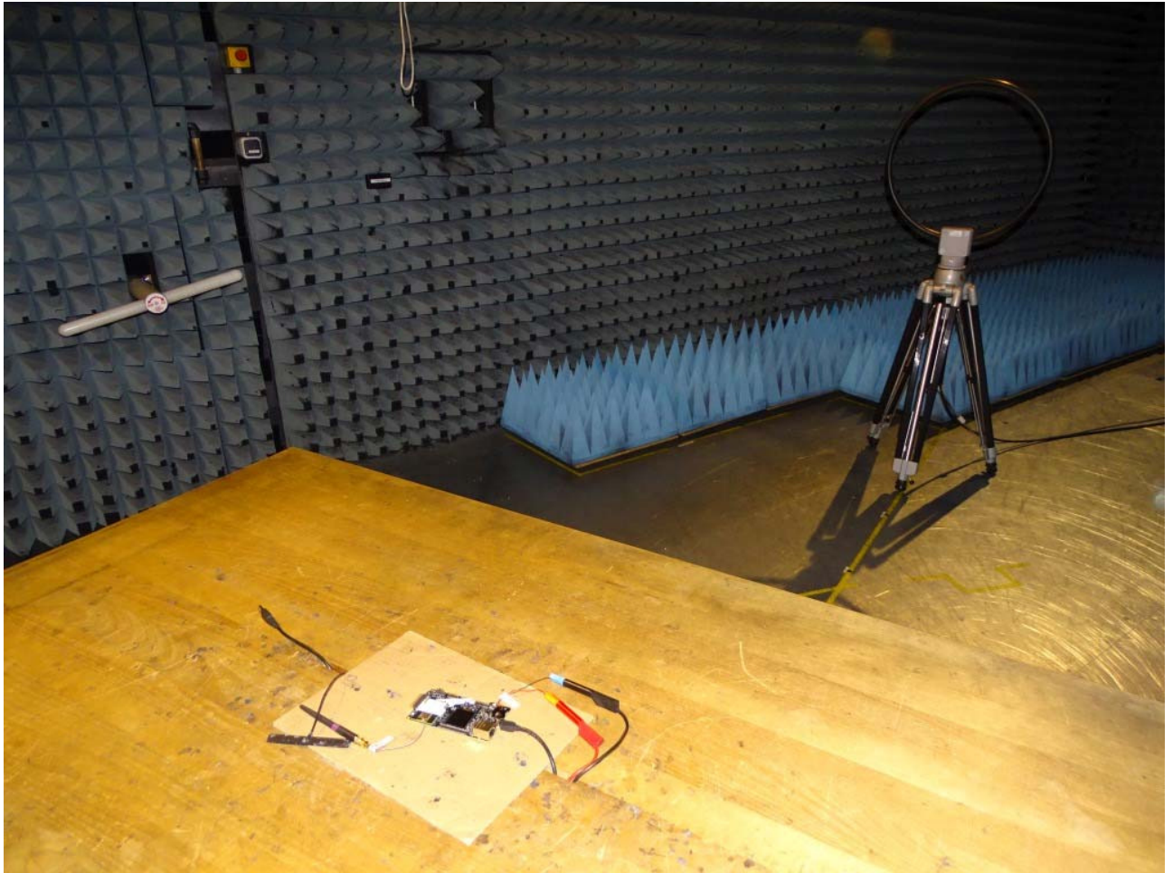
Photo 1: Test setup for radiated measurements below 30 MHz, side view
