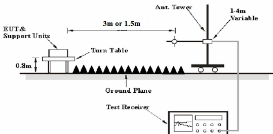
The radiated emission tests were performed in the 3 meters chamber, using the setup accordance with the ANSI C63.4-2003. The specification used was the FCC 15.209, and FCC 15.407 limits.
