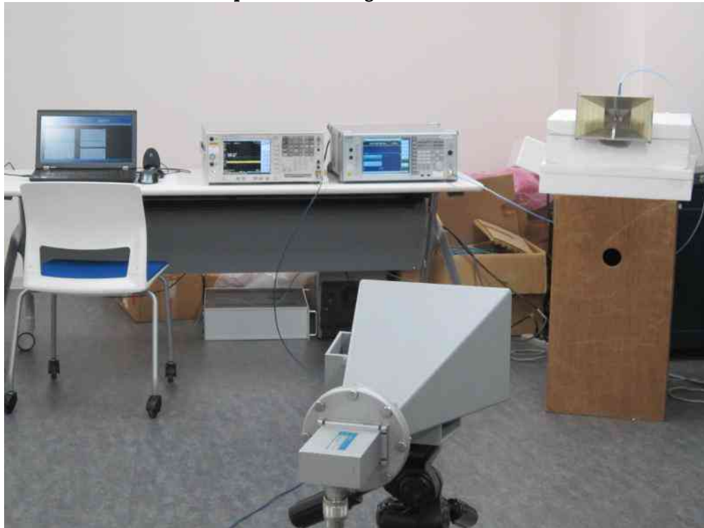
Test Setup for Generating the Radar Waveform
