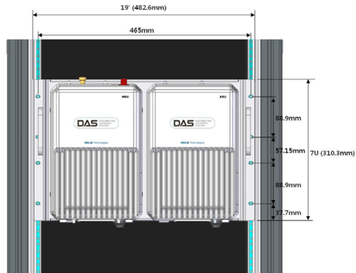
Figure 5.19 – ROU installation diagram for vertical rack
