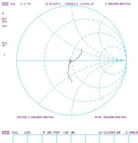
Impedance & Return-Loss Measurement Plot for Head TSL
