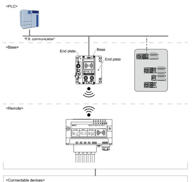
IO-Link devices: Pressure switch, digital flow switch, electro-pneumatic regulator, position sensor, SI unit (solenoid valve)
