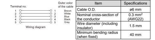
(3) Y junction connector for IO-Link
