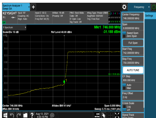
Plot 7-313. Band Edge Emission (745.9MHz to 746MHz) Plot (LTE_B13_5M+5M_2C_256QAM - Port 2)
