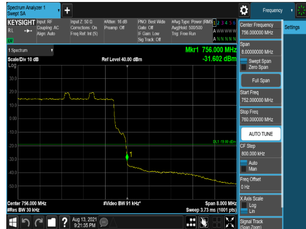
Plot 7-322. Band Edge Emission (756MHz to 756.1MHz) Plot (LTE_B13_10M+High_NB-lot(IB)+High_NB-lot(IB)_1C – Port 3)
