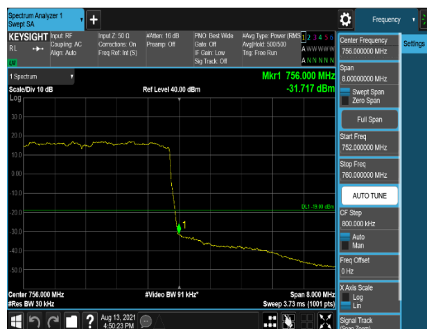
Plot 7-314. Band Edge Emission (756MHz to 756.1MHz) Plot (LTE_B13_5M+5M_2C_16QAM - Port 3)
