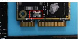
This part of the circuit is reserved. This part of the component is removable, This has no effect on module performance.
