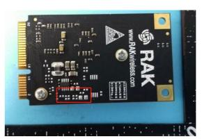
This part of the circuit is reserved. This part of the component is removable, This has no effect on module performance.
