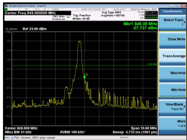
LTE Band 5 QPSK 5MHz CH-High 100%RB
