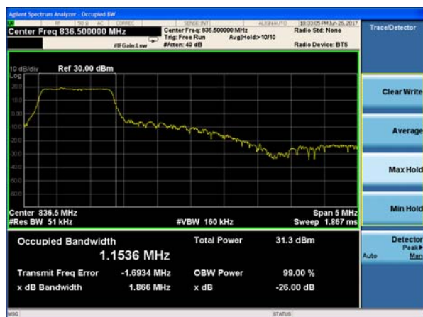
LTE Band 5 QPSK 5MHz CH-Middle
