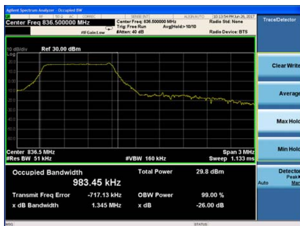
LTE Band 5 16QAM 5MHz CH-Middle
