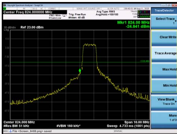
LTE Band 5 16QAM 10MHz CH-Low 1RB
