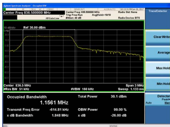
LTE Band 5 QPSK 5MHz CH-Middle
