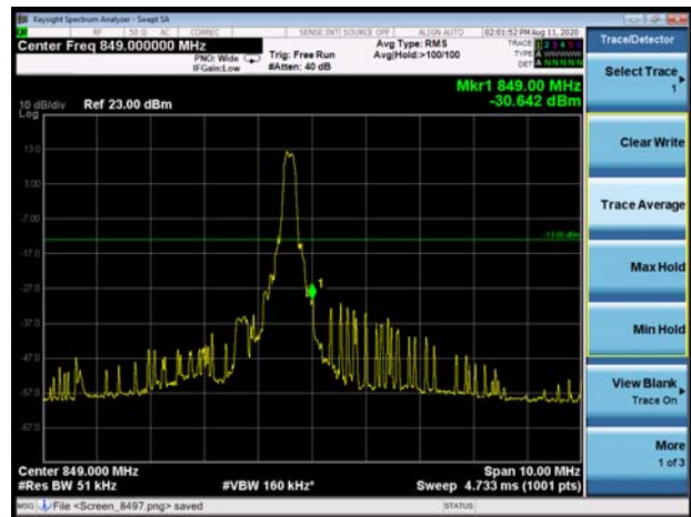
LTE Band 5 QPSK 5MHz CH-High 1RB
