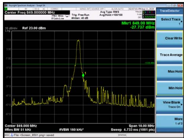
LTE Band 5 QPSK 5MHz CH-High 100%RB
