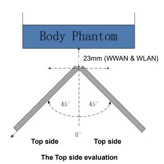
Based on the above evaluation, we come to the conclusion that the sensor triggering is not released and normal maximum output power is not restored within the  $\pm 45^{\circ}$  range at the smallest sensor triggering test distance declared by manufacturer.
