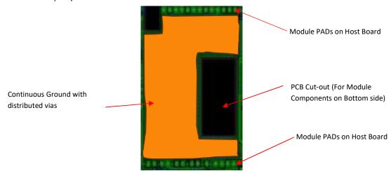
The top layer (underneath the module) of the host PCB must be ground with as many GND vias as possible.
