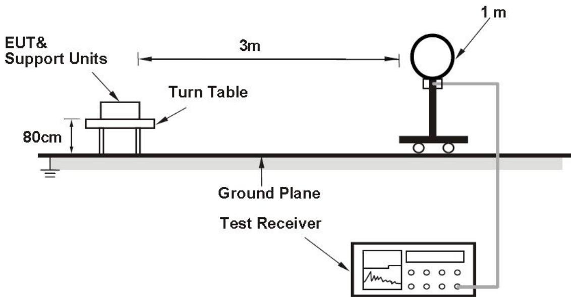
For Radiated emission 30MHz to 1GHz
