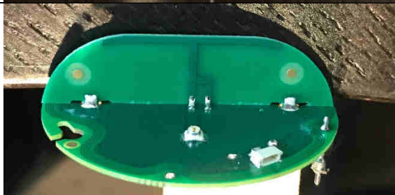
Antenna element PCB trace and feed point
