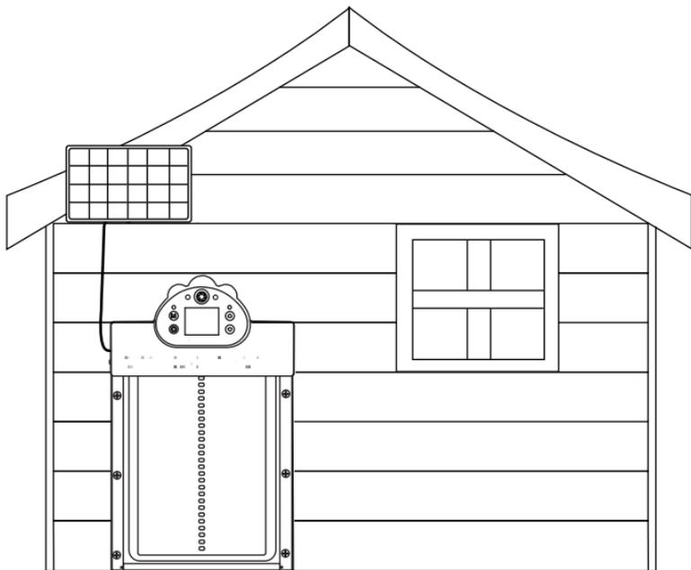
④ Connect the solar panel with a Type-C charging cable and place the solar panel in a suitable location.
