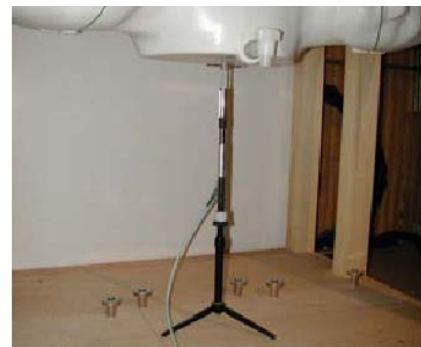
Figure 11.1 Dipole Verification Test Setup Diagram & Photo
