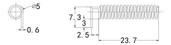
Antenna material : spring steel Antenna wire diameter:0.6mm Number of antenna coils:16circle Antenna gain: 0dbi
