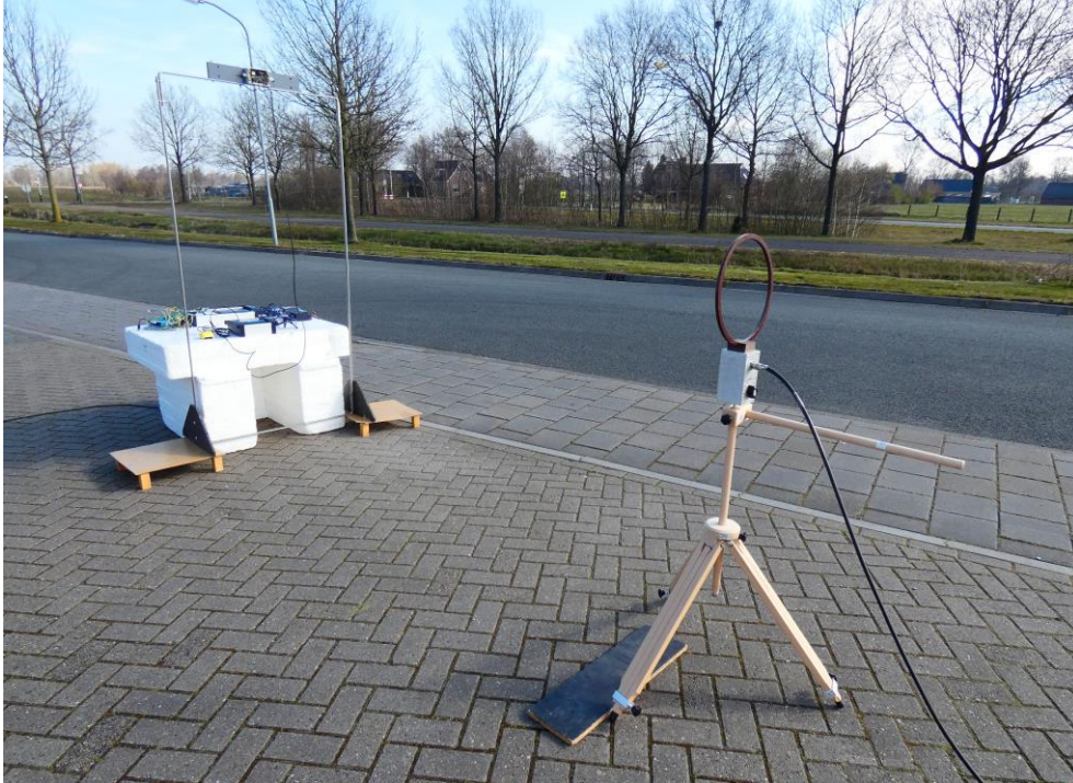
Setup EUT with Single Walk Through antenna, @3m Axial (X-orientation)
