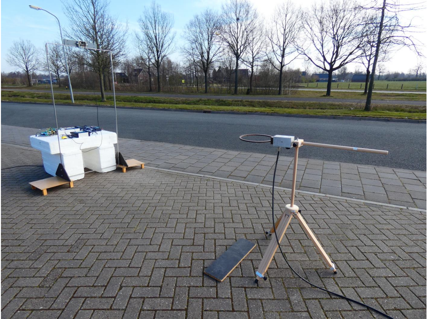
Setup EUT with Single Walk Through antenna, @3m Axial (Z-orientation)
