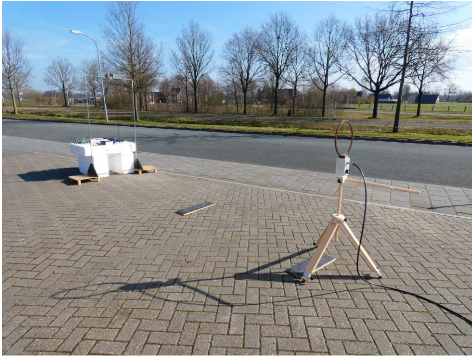
Setup EUT with Single Walk Through antenna, @5m (X-orientation shown)
