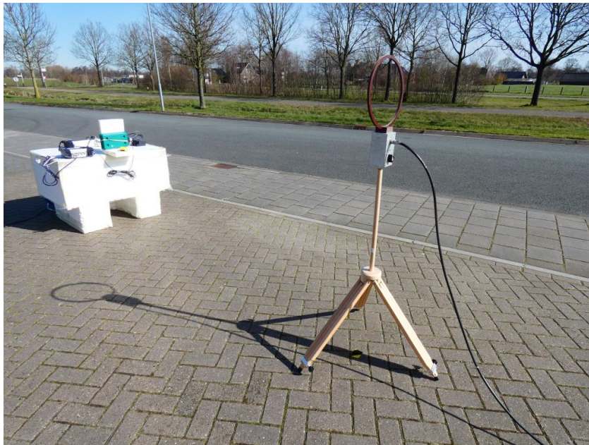
Setup EUT with VP6012 antenna @3m
