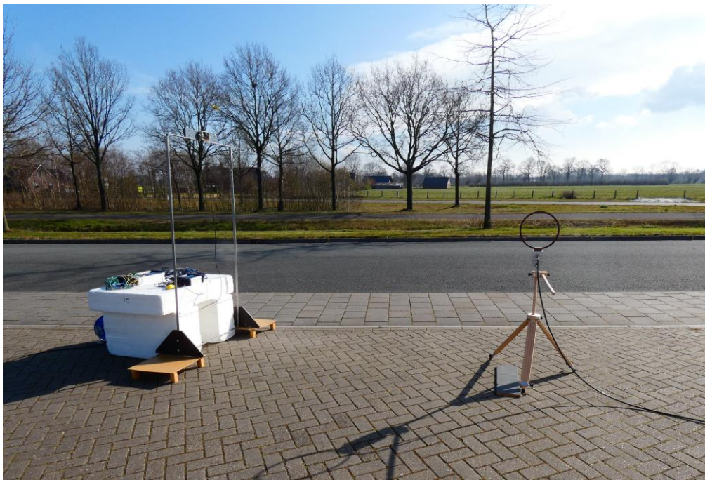
Setup EUT with Single Walk Through antenna, @3m Axial (Y-orientation)
