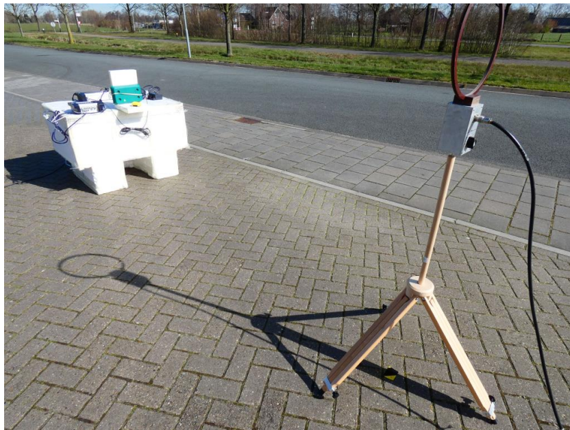
Setup EUT with VP6012 antenna @5m
