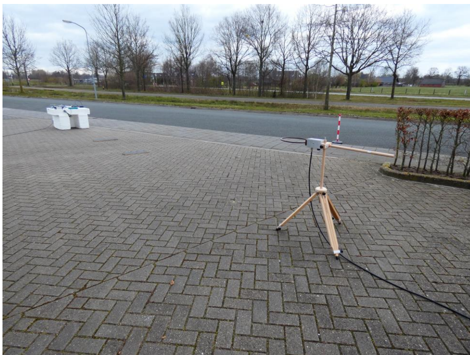
Setup EUT with VP6012 antenna @10m (Z-orientation shown)
