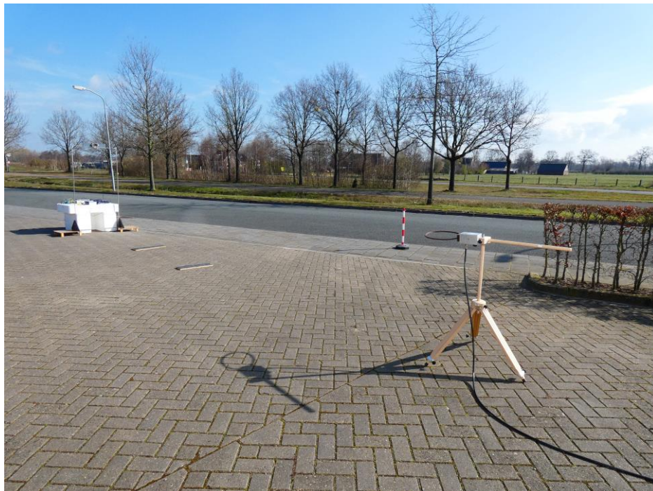
Setup EUT with Single Walk Through antenna, @10m (Z-orientation shown)
