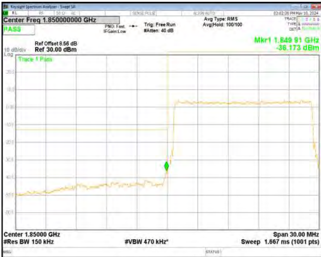
Band25 16QAM BW=5MHz Channel=26665 RB Size=25 Position=#0
