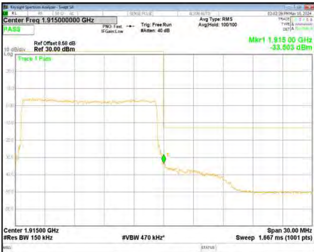
Band25 QPSK BW=15MHz Channel=26115 RB Size=75 Position=#0
