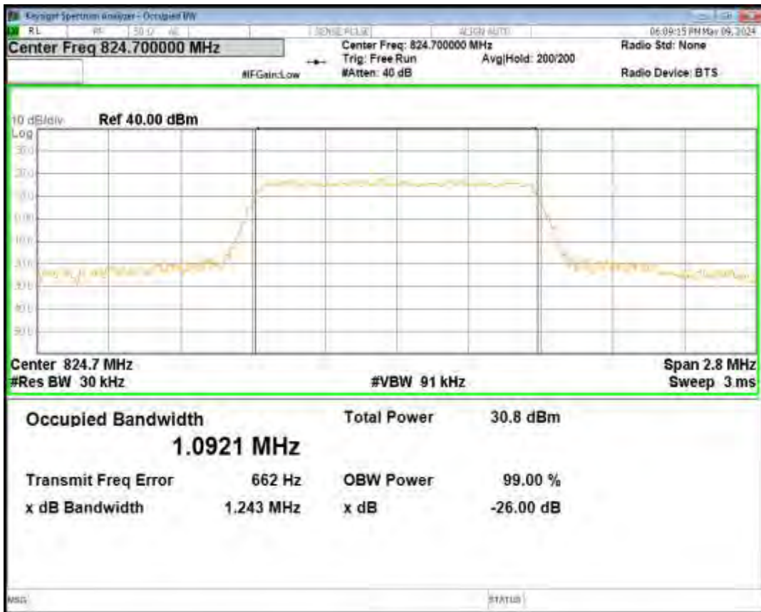
Band5 16QAM BW=5MHz Channel=20625 RB Size=25 Position=#0
