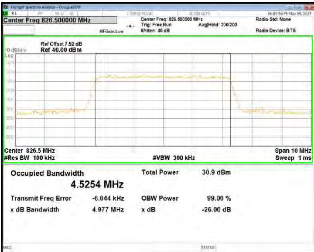
Band5 QPSK BW=5MHz Channel=20525 RB Size=25 Position=#0
