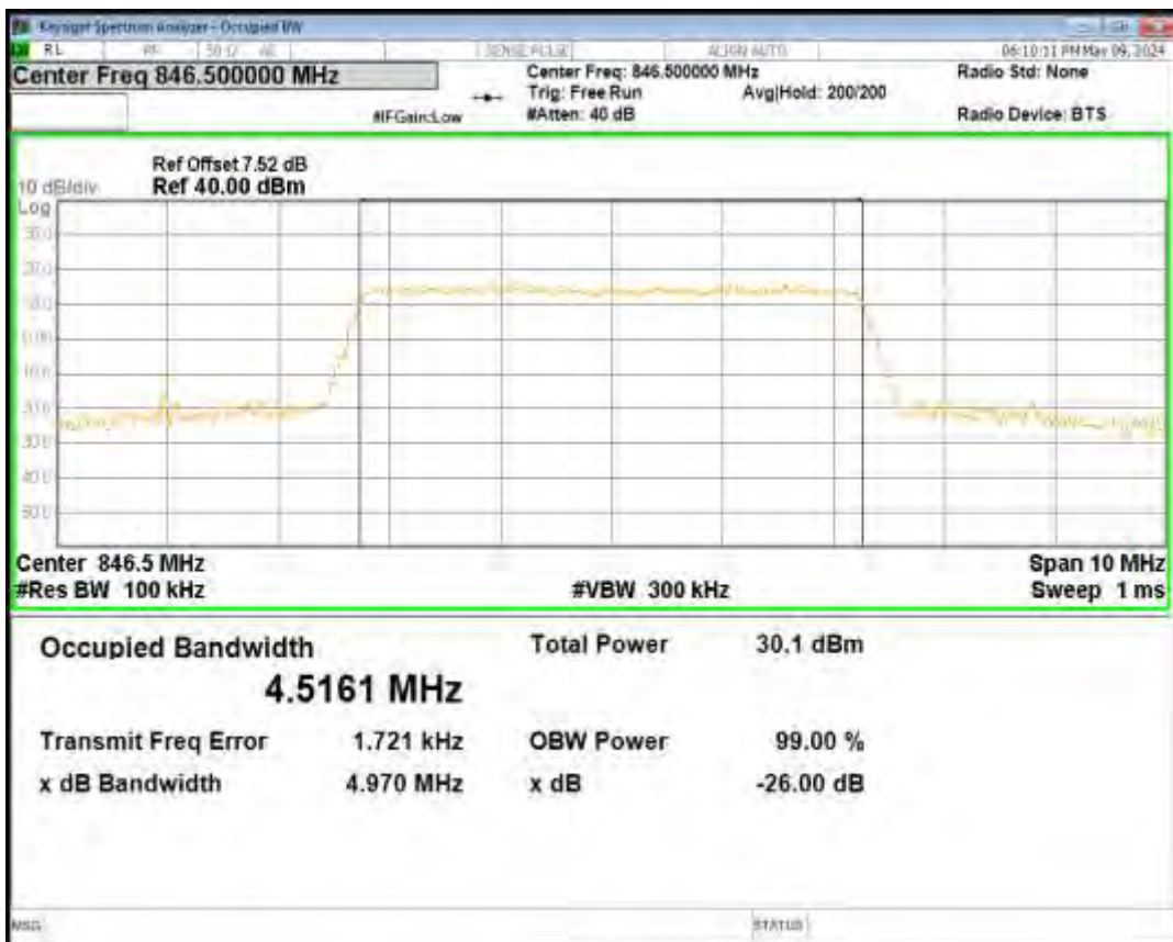
Band5 16QAM BW=5MHz Channel=20525 RB Size=25 Position=#0
