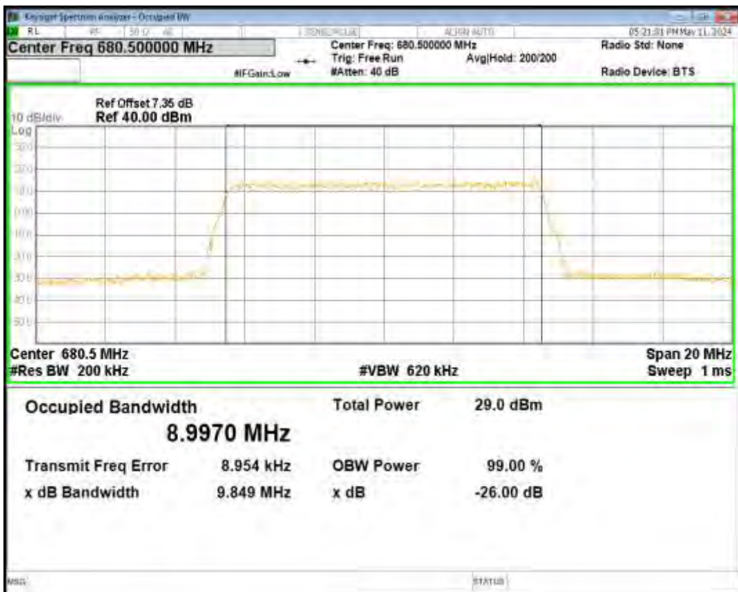
Band71 16QAM BW=10MHz Channel=133422 RB Size=50 Position=#0
