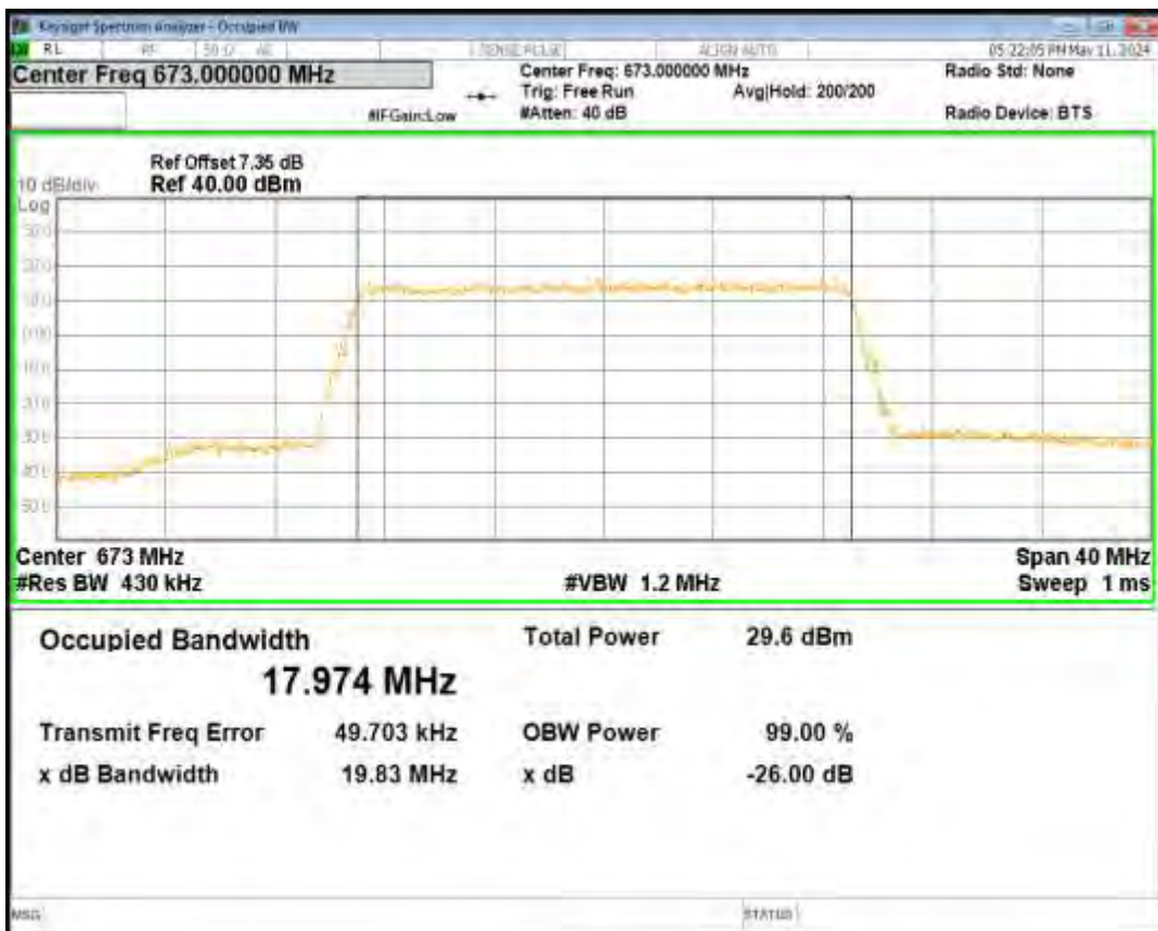
Band71 QPSK BW=15MHz Channel=133397 RB Size=75 Position=#0
