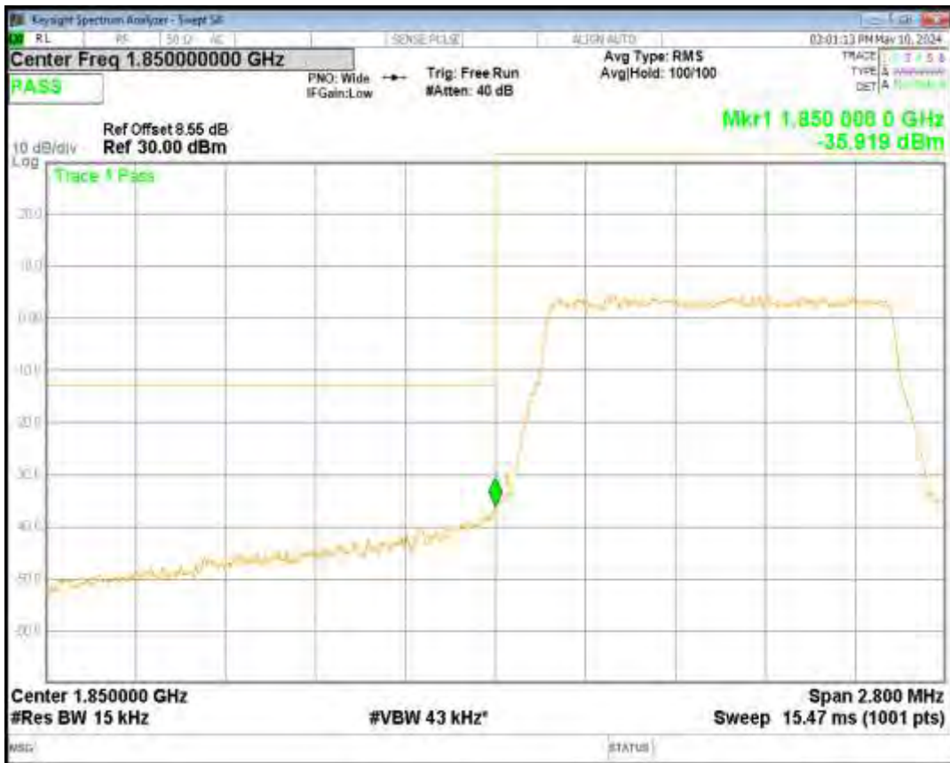
Band25 16QAM BW=1.4MHz Channel=26683 RB Size=6 Position=#0
