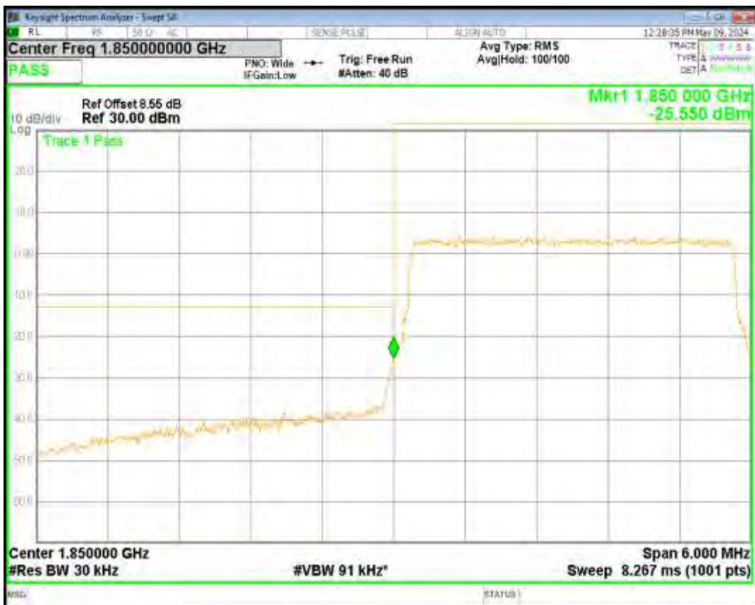
Band2 16QAM BW=20MHz Channel=19100 RB Size=100 Position=#0
