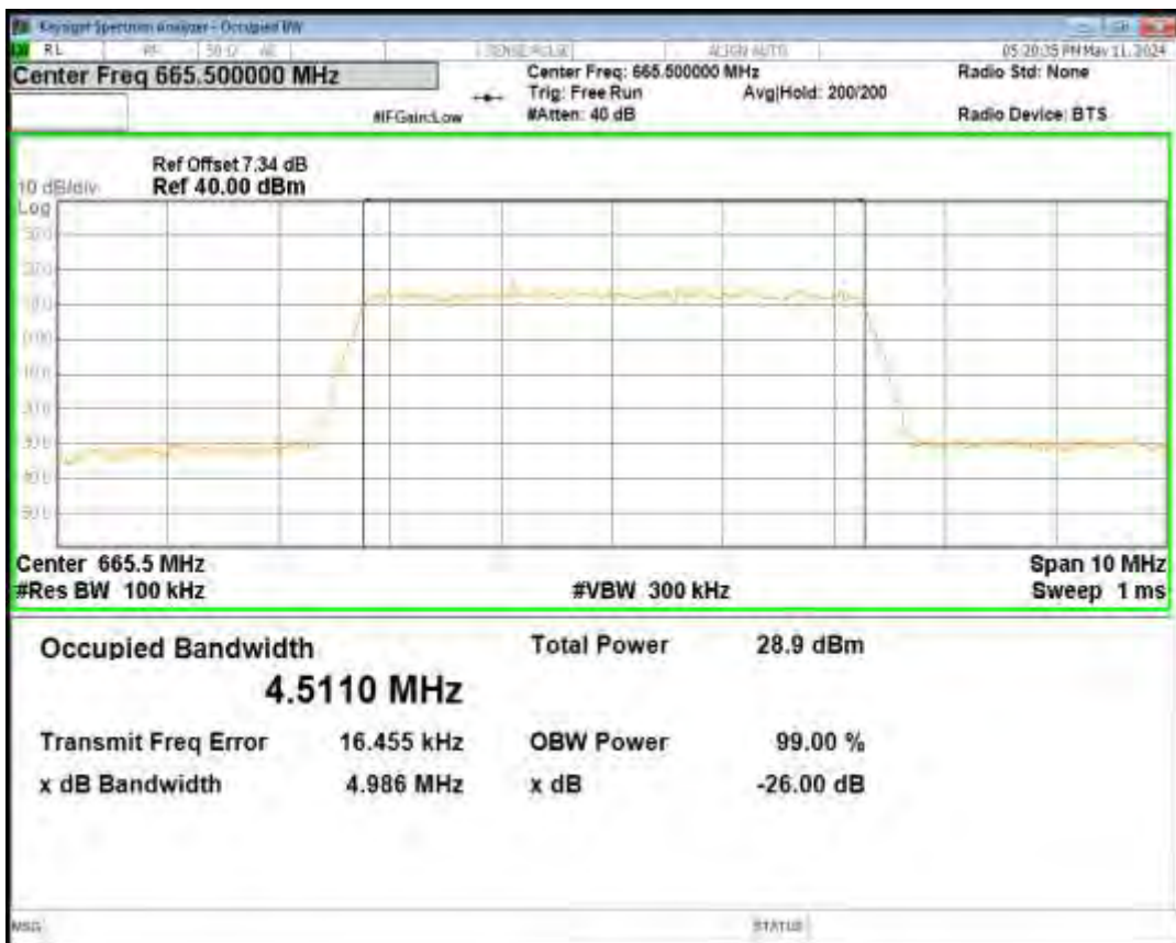
Band71 QPSK BW=5MHz Channel=133147 RB Size=25 Position=#0
