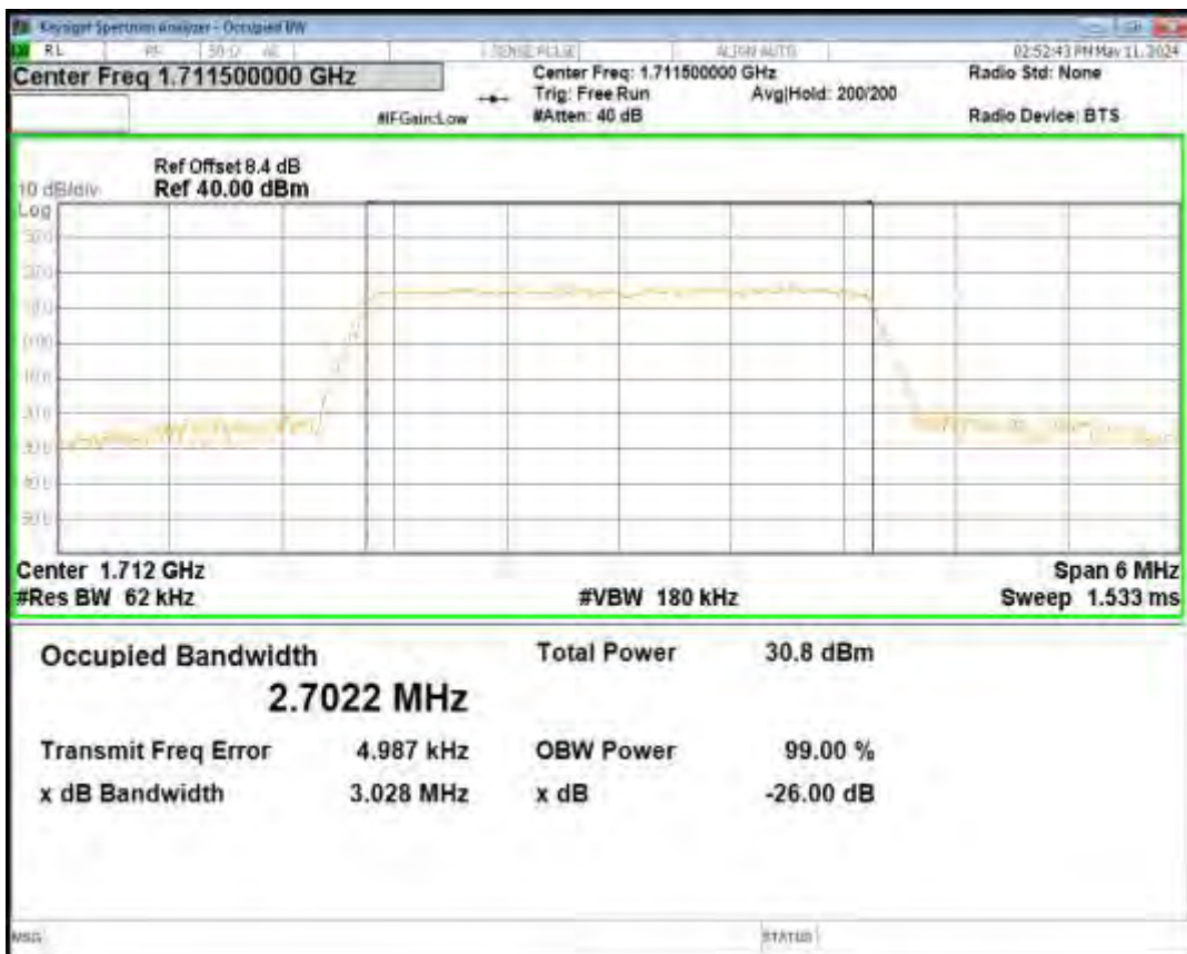
Band66 16QAM BW=20MHz Channel=132572 RB Size=100 Position=#0
