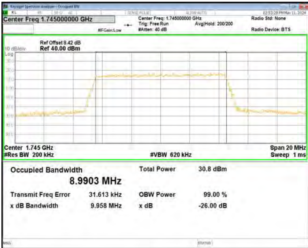
Band66 QPSK BW=5MHz Channel=132322 RB Size=25 Position=#0
