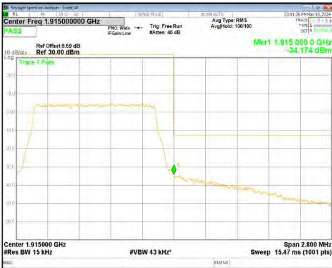
Band25 QPSK BW=1.4MHz Channel=26047 RB Size=6 Position=#0
