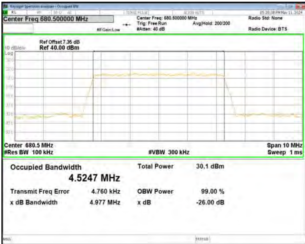
Band71 16QAM BW=5MHz Channel=133297 RB Size=25 Position=#0
