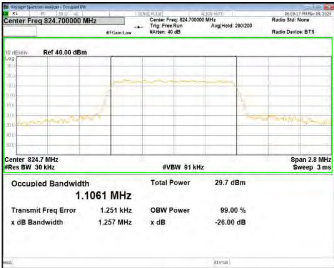
Band5 16QAM BW=1.4MHz Channel=20525 RB Size=6 Position=#0
