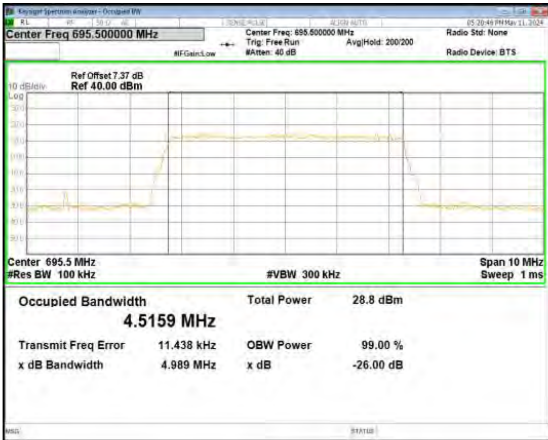
Band71 QPSK BW=10MHz Channel=133422 RB Size=50 Position=#0
