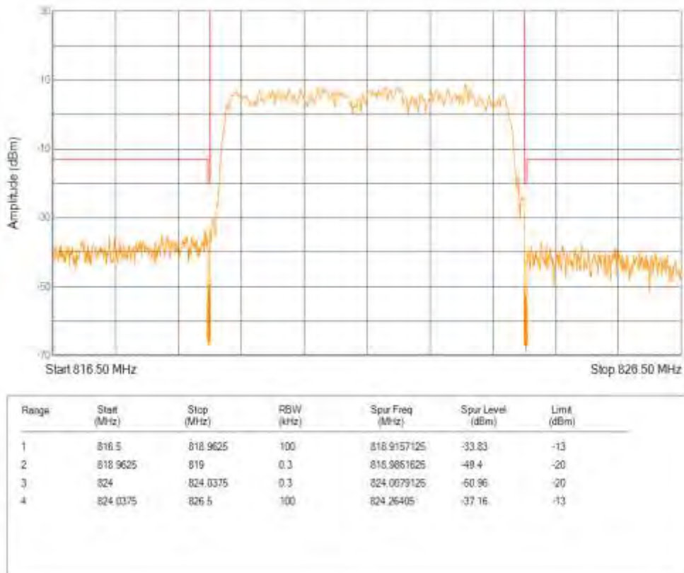
Band26(824-849) 16QAM BW=1.4MHz Channel=26797 RB Size=6 Position=#0
