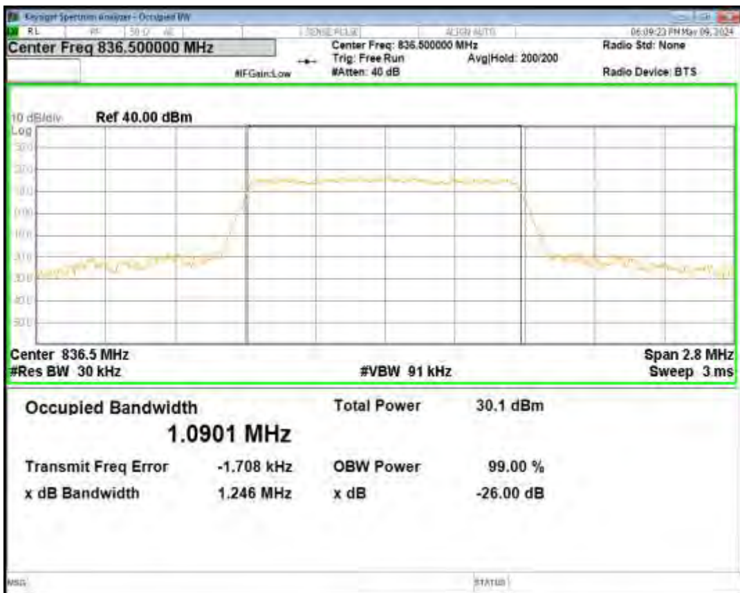
Band5 16QAM BW=1.4MHz Channel=20643 RB Size=6 Position=#0
