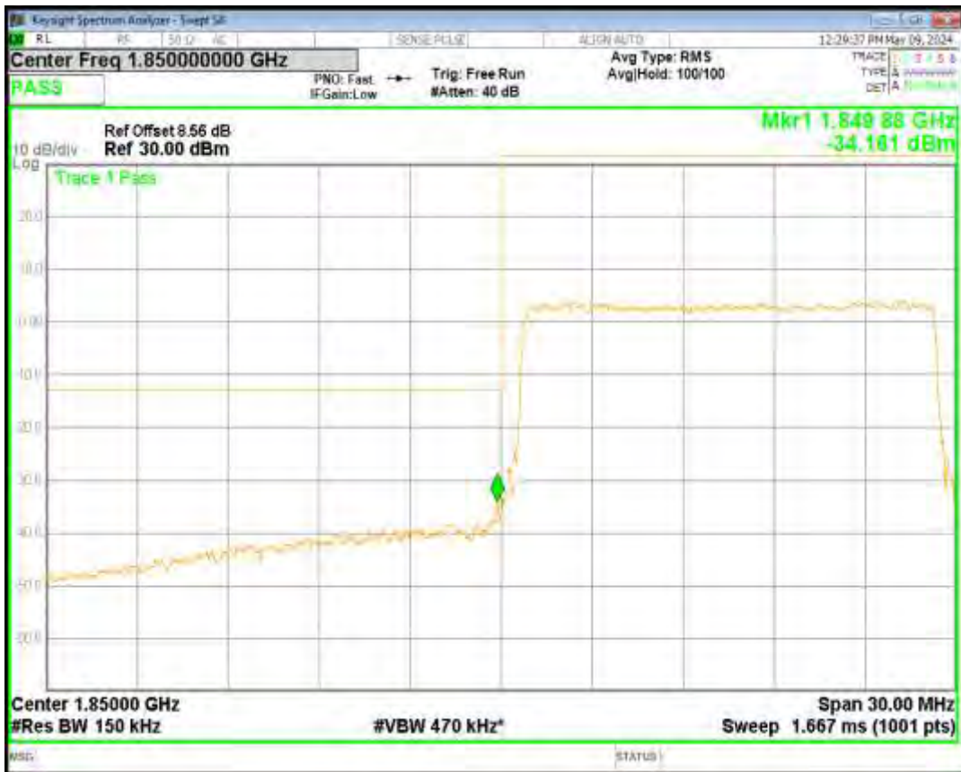
Band2 16QAM BW=15MHz Channel=19125 RB Size=75 Position=#0
