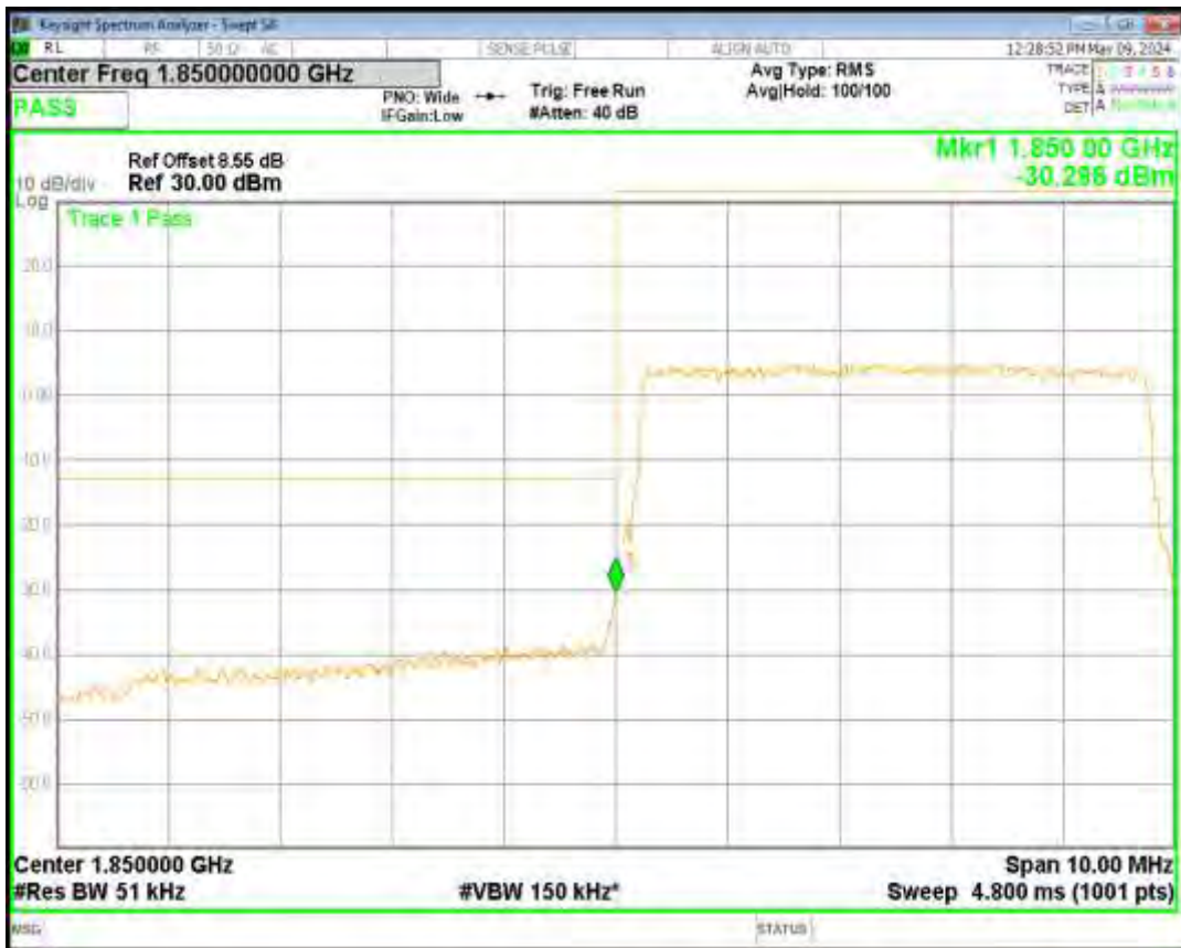
Band2 QPSK BW=15MHz Channel=18675 RB Size=75 Position=#0
