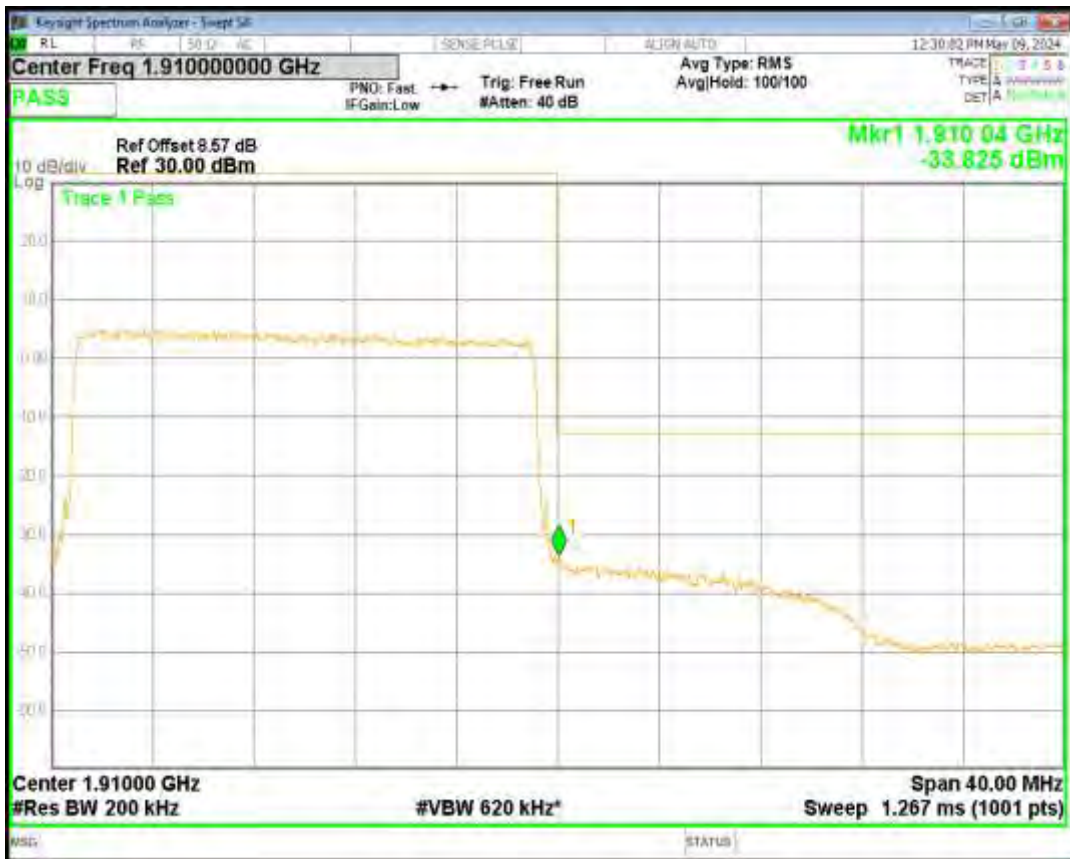
Band2 QPSK BW=3MHz Channel=18615 RB Size=15 Position=#0
