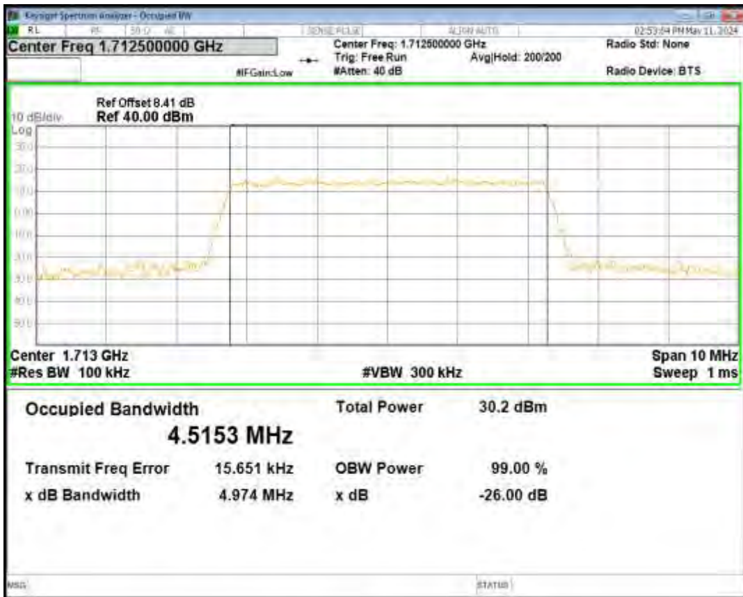
Band66 16QAM BW=3MHz Channel=132657 RB Size=15 Position=#0
