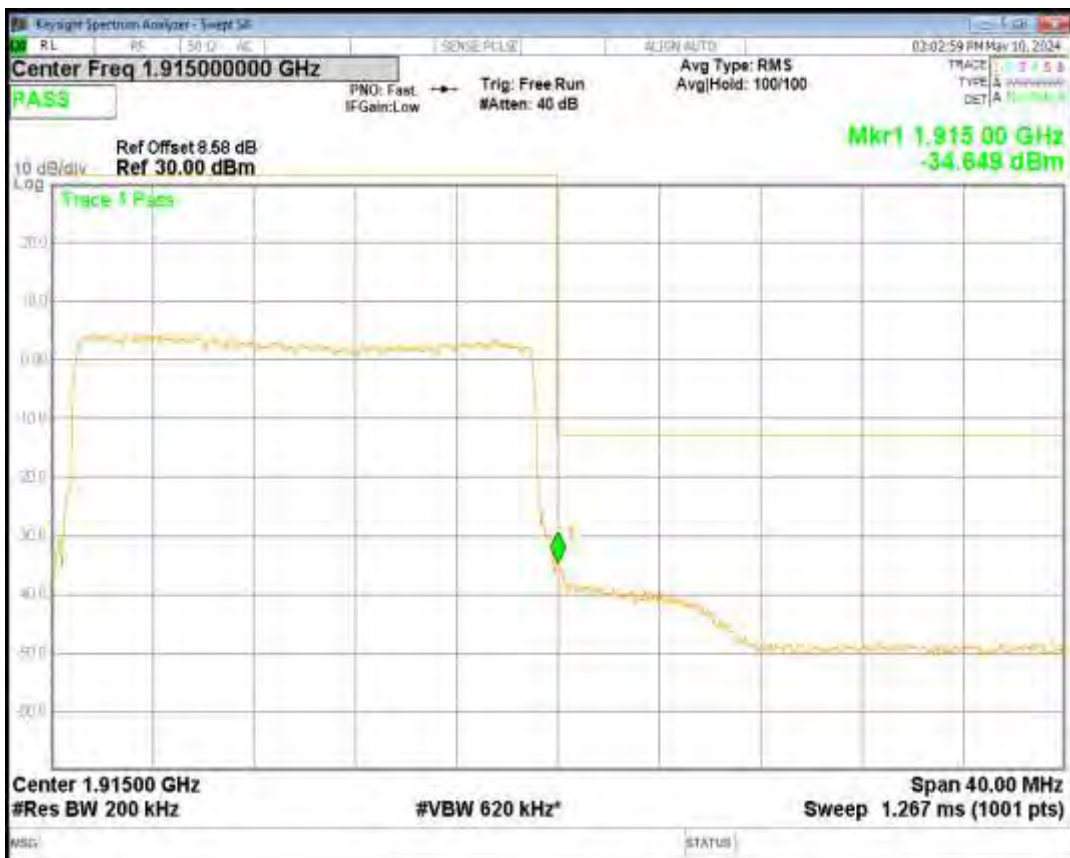
Band25 QPSK BW=20MHz Channel=26140 RB Size=100 Position=#0
