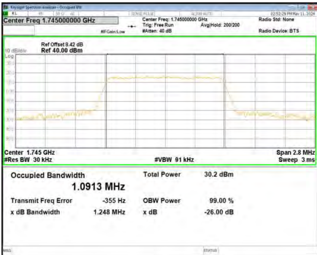
Band66 16QAM BW=1.4MHz Channel=132665 RB Size=6 Position=#0
