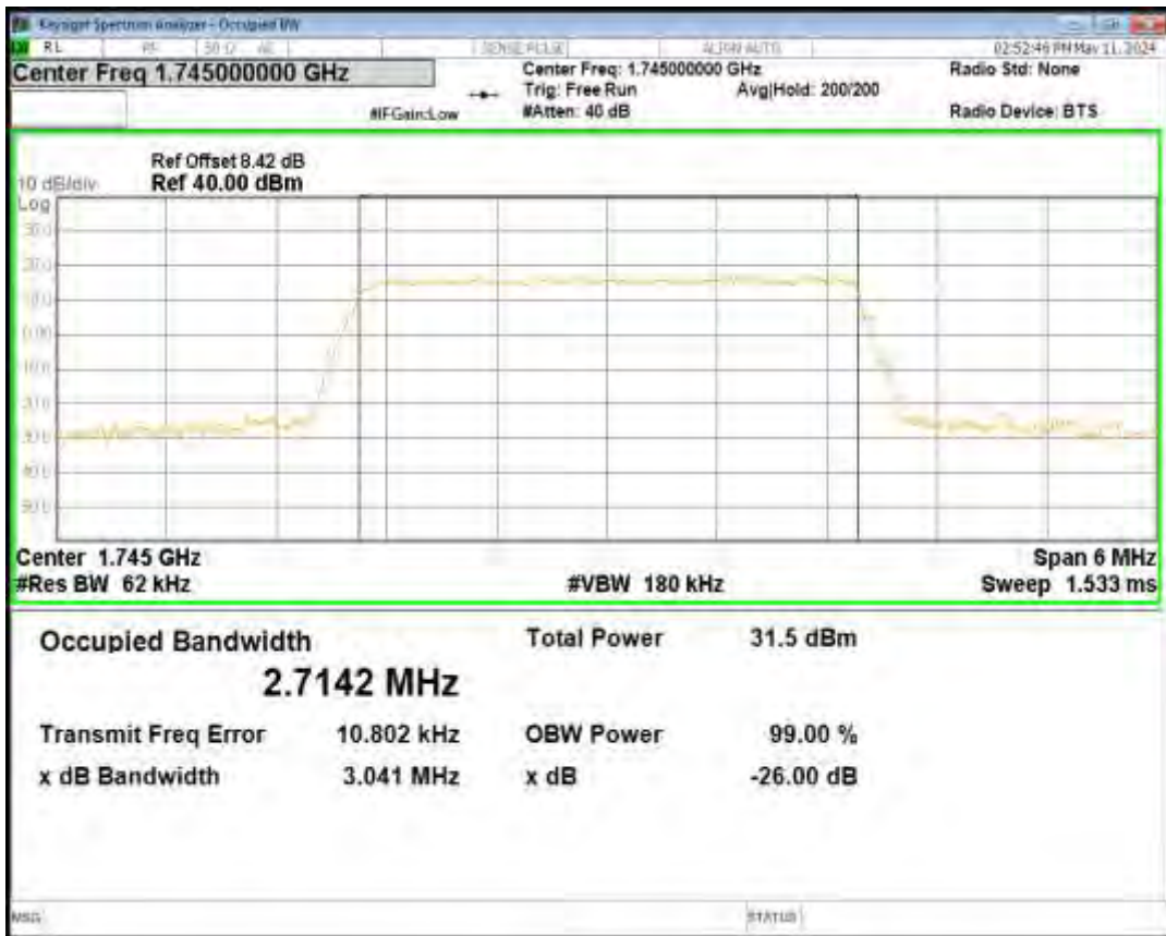
Band66 QPSK BW=3MHz Channel=132657 RB Size=15 Position=#0
