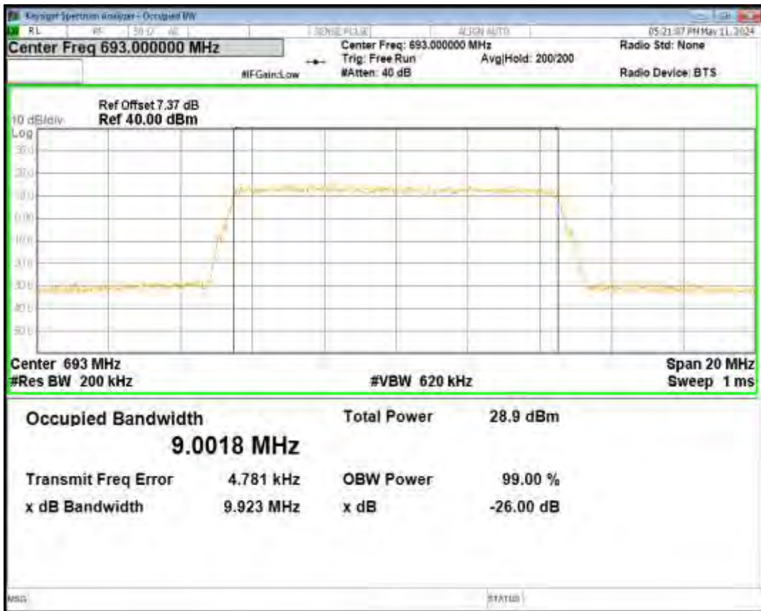
Band71 16QAM BW=15MHz Channel=133197 RB Size=75 Position=#0
