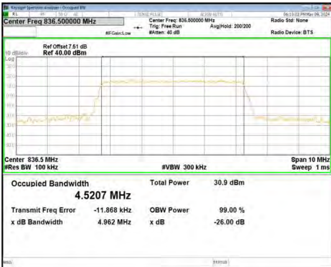
Band5 QPSK BW=5MHz Channel=20625 RB Size=25 Position=#0
