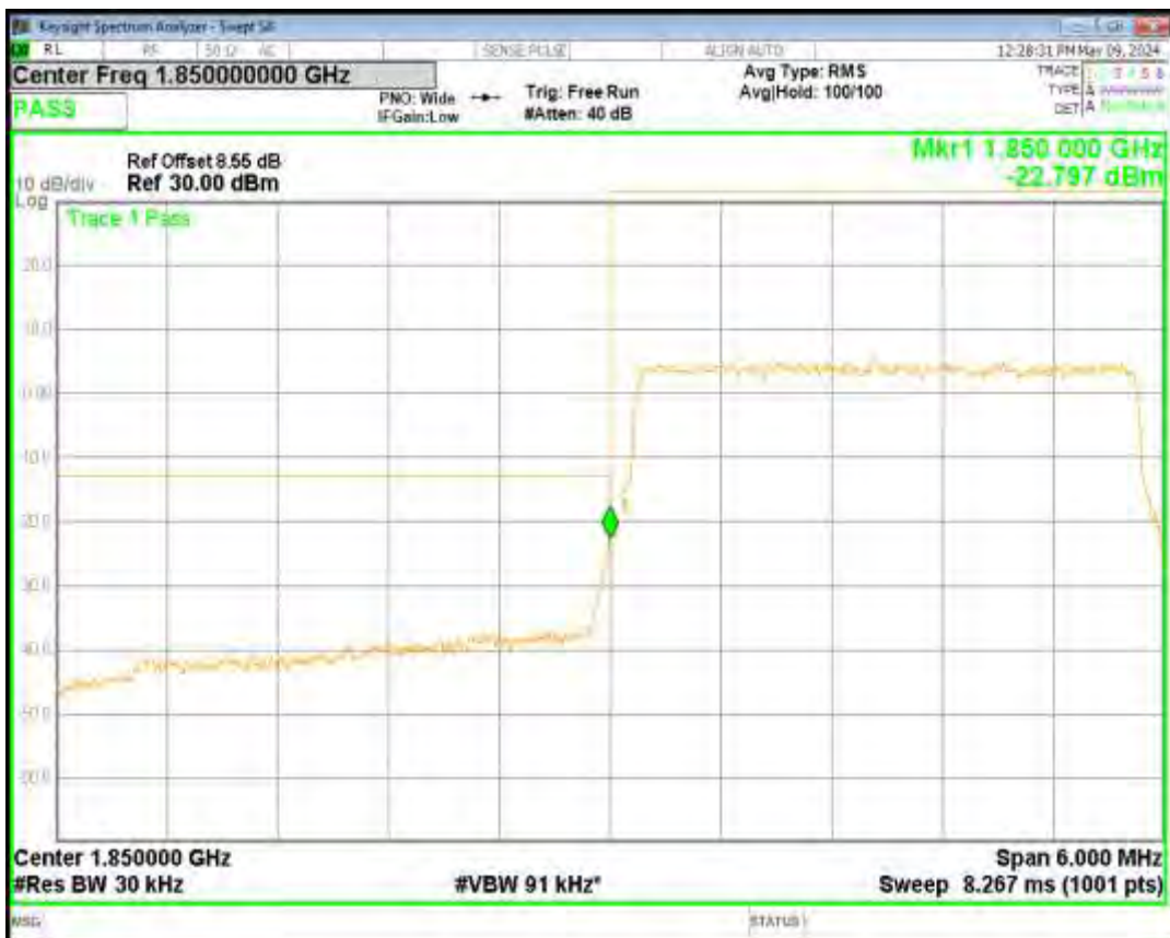
Band2 QPSK BW=3MHz Channel=19185 RB Size=15 Position=#0
