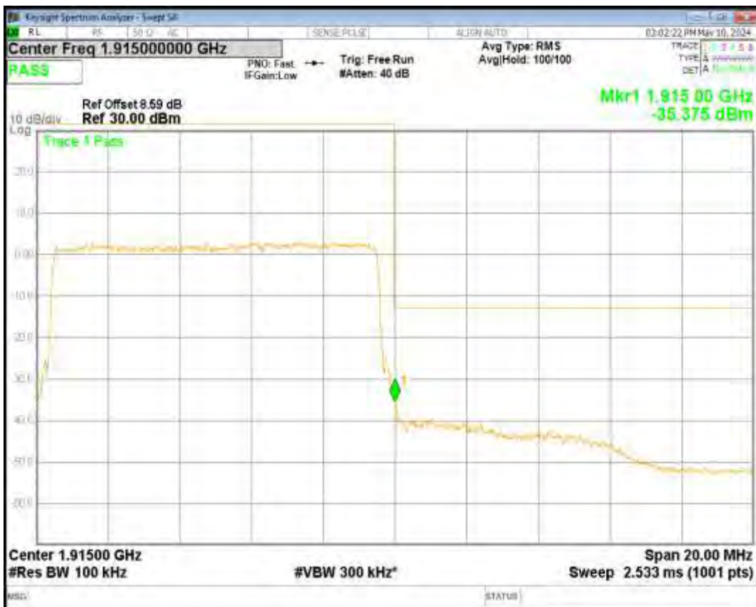
Band25 16QAM BW=15MHz Channel=26115 RB Size=75 Position=#0
