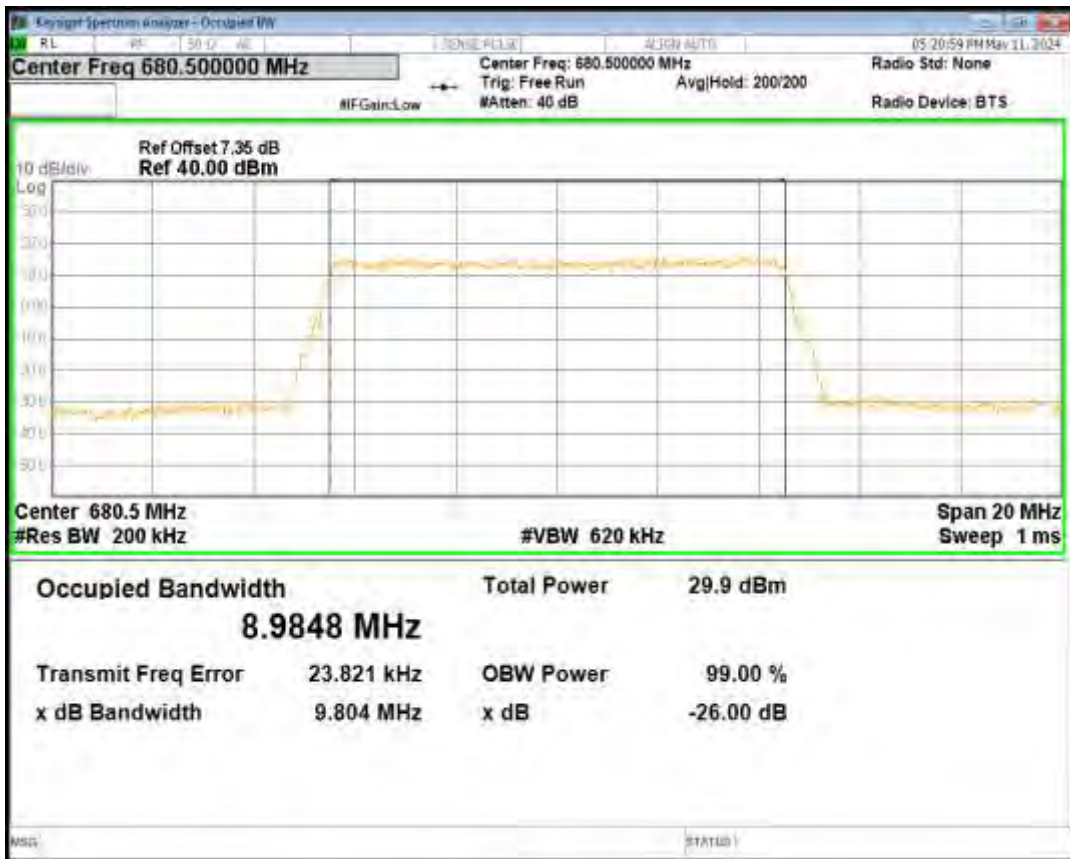
Band71 QPSK BW=10MHz Channel=133172 RB Size=50 Position=#0
