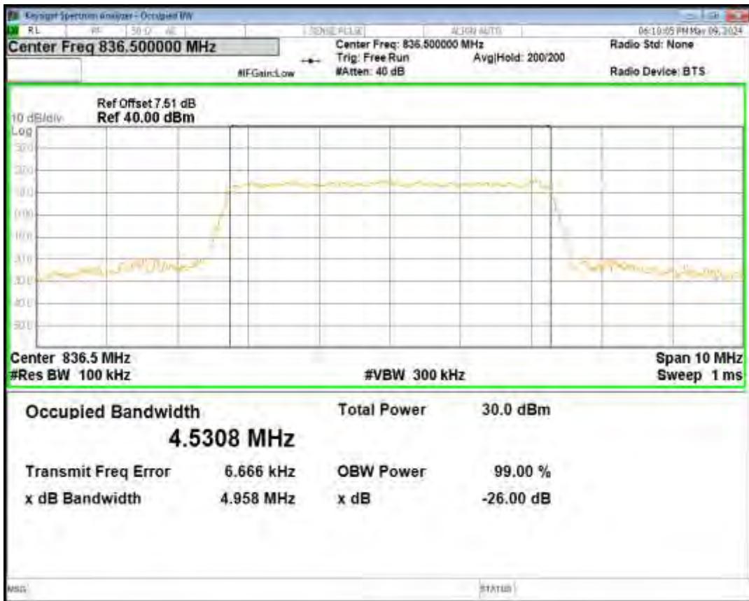
Band5 QPSK BW=1.4MHz Channel=20525 RB Size=6 Position=#0
