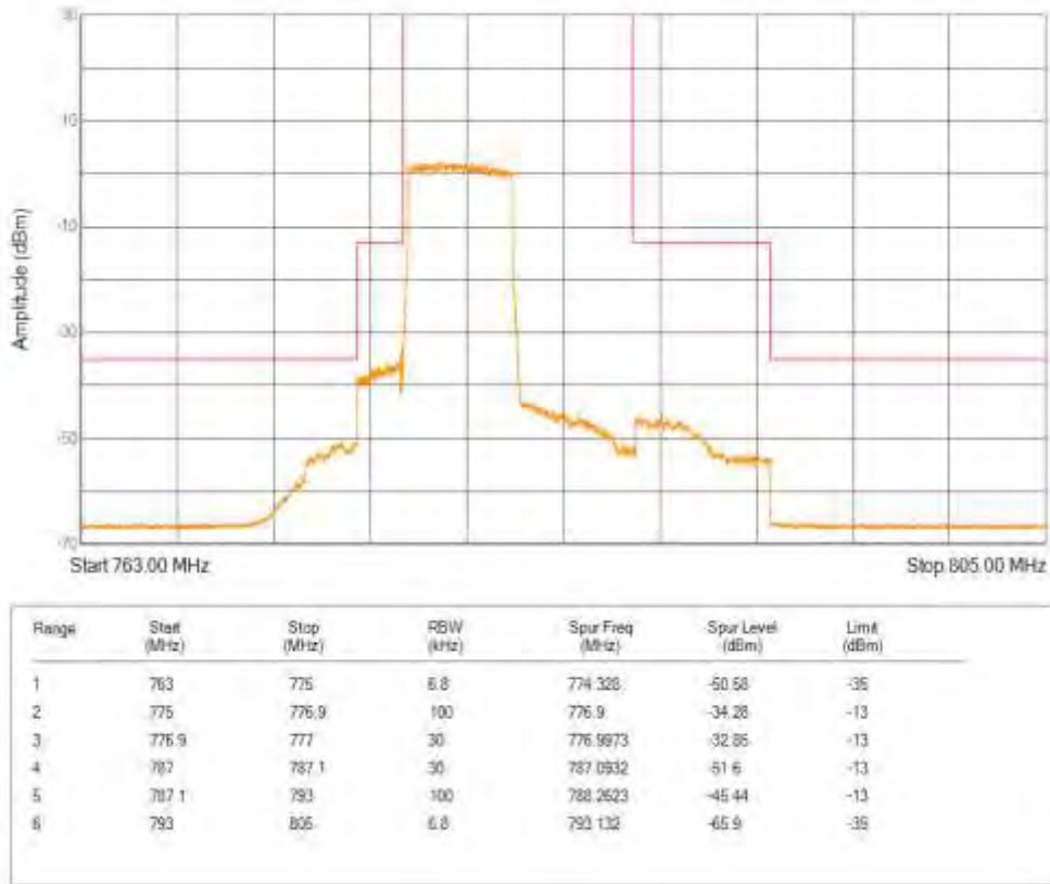
Band13 QPSK BW=5MHz Channel=23255 RB Size=25 Position=#0
