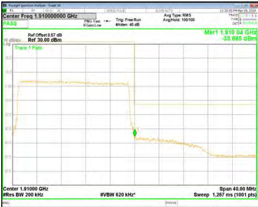
Band2 16QAM BW=3MHz Channel=19185 RB Size=15 Position=#0
