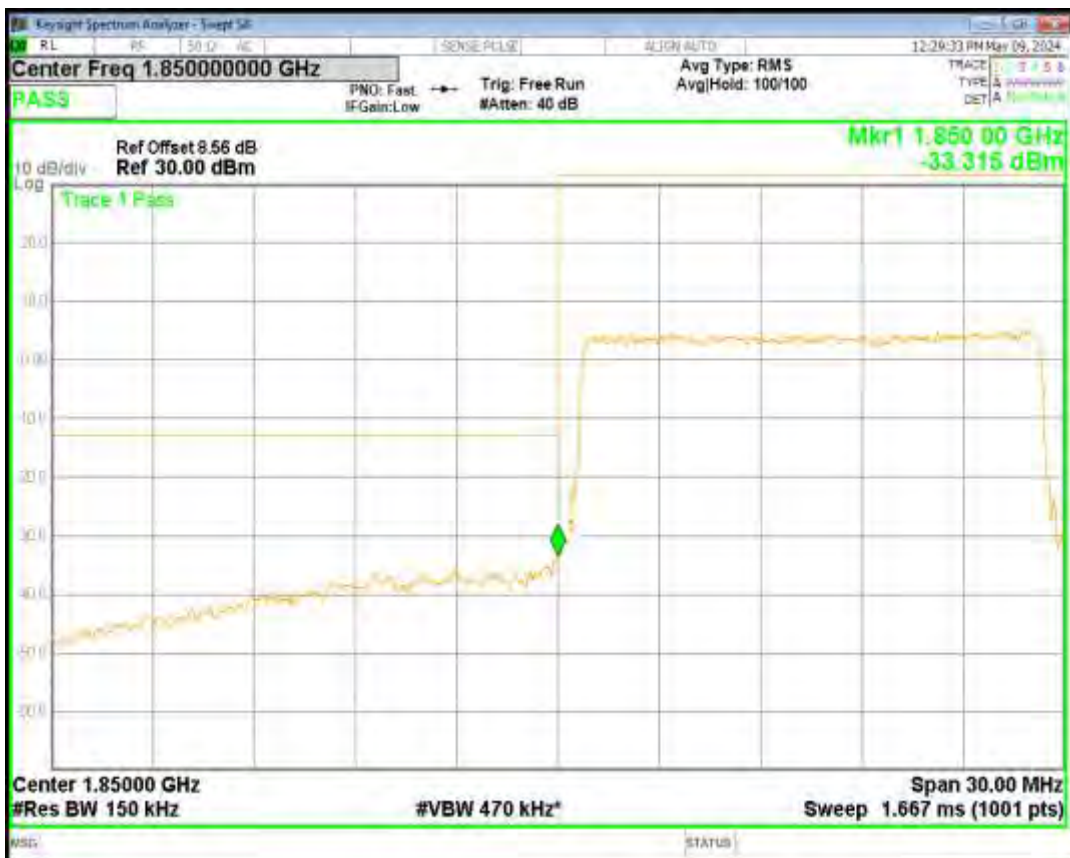
Band2 QPSK BW=15MHz Channel=19125 RB Size=75 Position=#0
