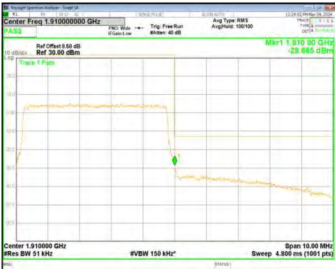
Band25 16QAM BW=1.4MHz Channel=26047 RB Size=6 Position=#0
