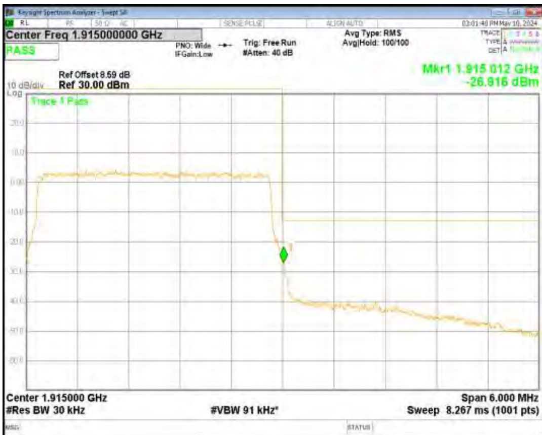
Band25 QPSK BW=3MHz Channel=26055 RB Size=15 Position=#0
