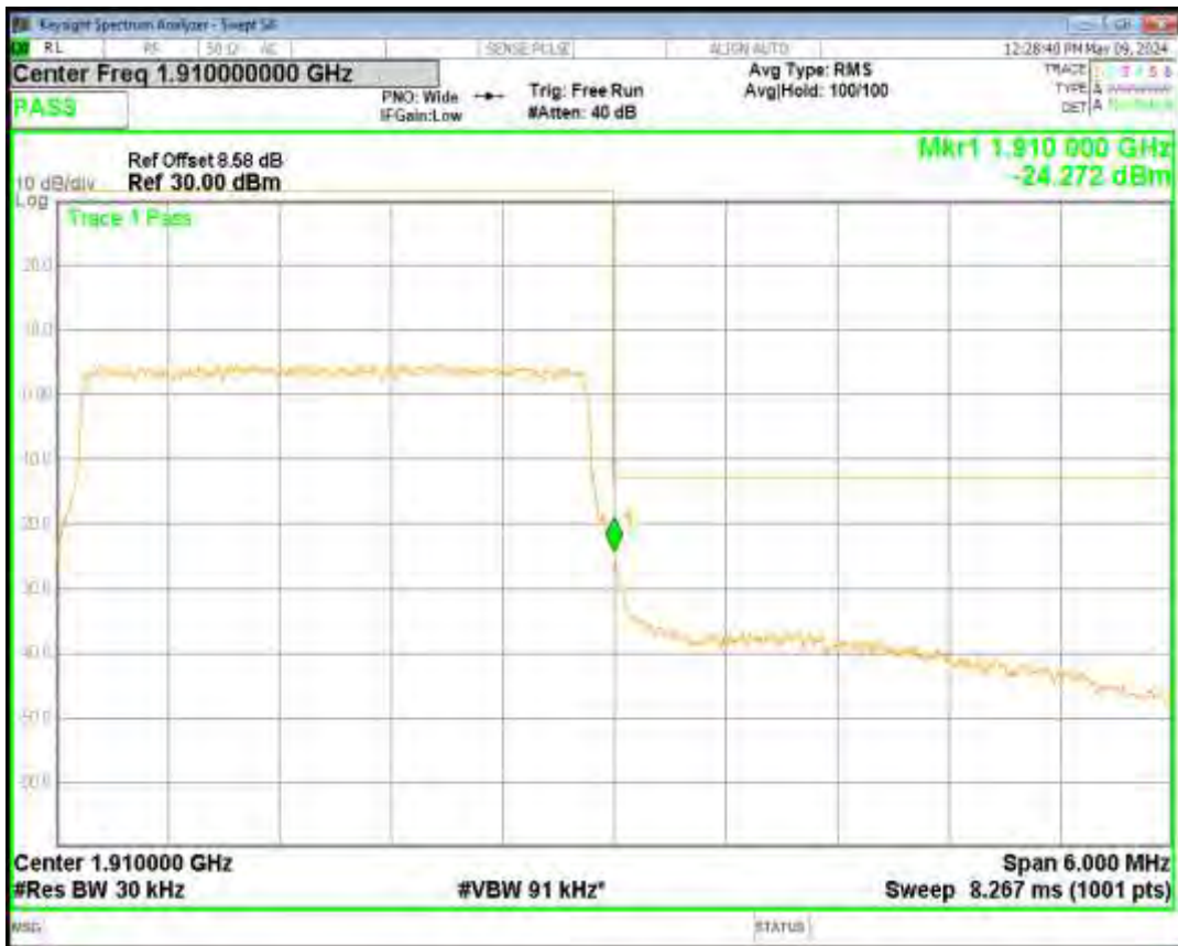
Band2 QPSK BW=5MHz Channel=19175 RB Size=25 Position=#0
