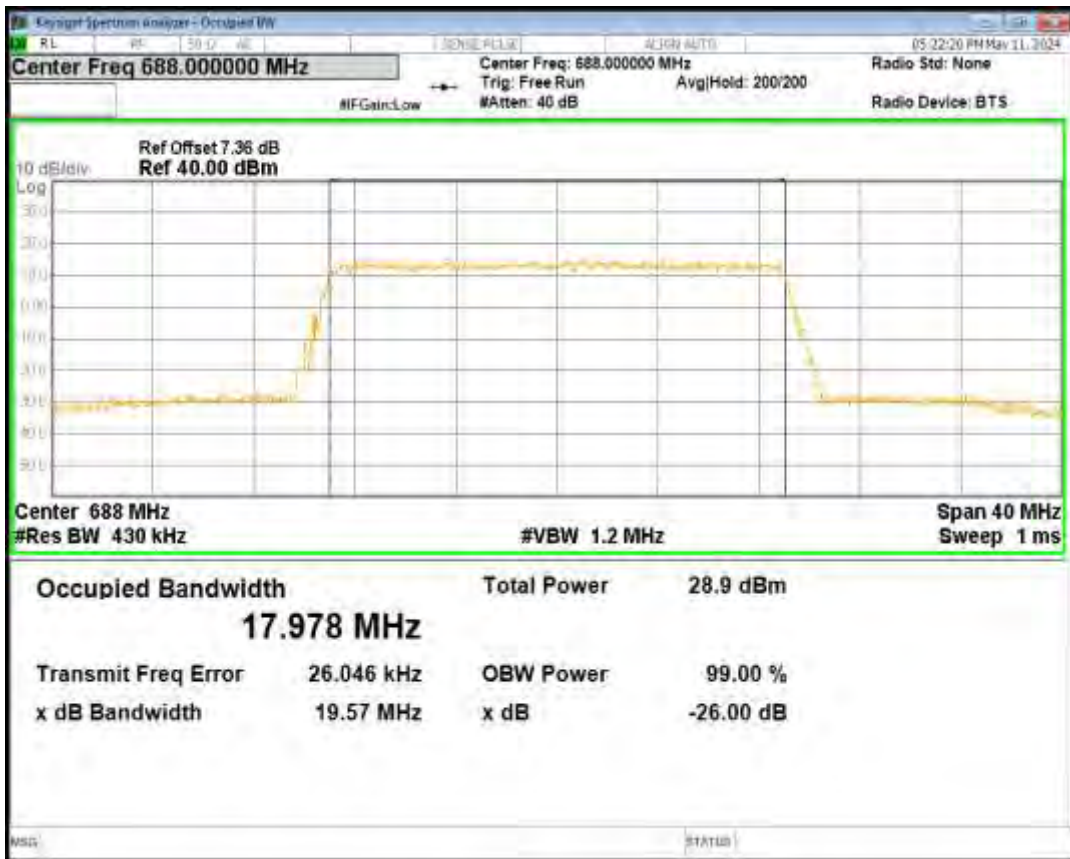
Band71 16QAM BW=5MHz Channel=133147 RB Size=25 Position=#0
