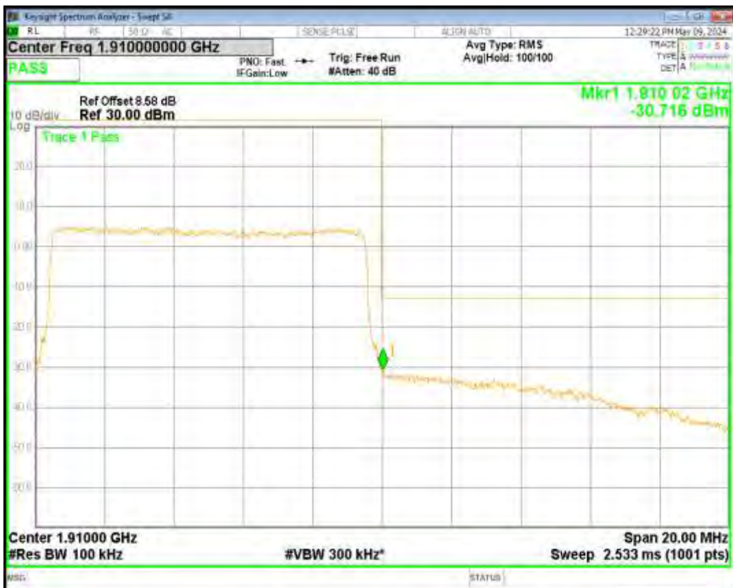
Band2 QPSK BW=5MHz Channel=18625 RB Size=25 Position=#0
