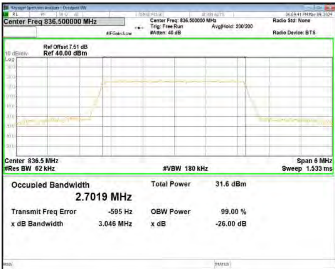
Band5 QPSK BW=3MHz Channel=20635 RB Size=15 Position=#0
