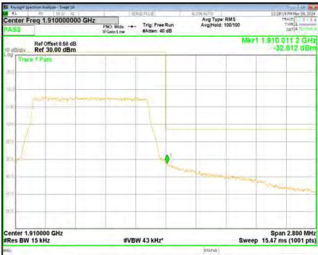
Band2 QPSK BW=1.4MHz Channel=18607 RB Size=6 Position=#0
