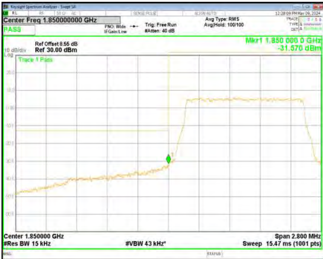
Band2 16QAM BW=5MHz Channel=18625 RB Size=25 Position=#0
