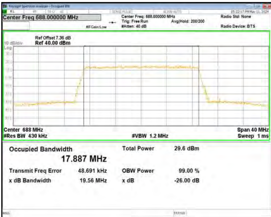
Band71 QPSK BW=20MHz Channel=133297 RB Size=100 Position=#0
