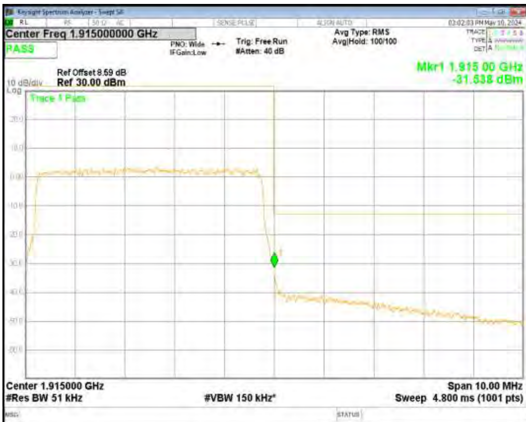
Band25 QPSK BW=10MHz Channel=26090 RB Size=50 Position=#0
