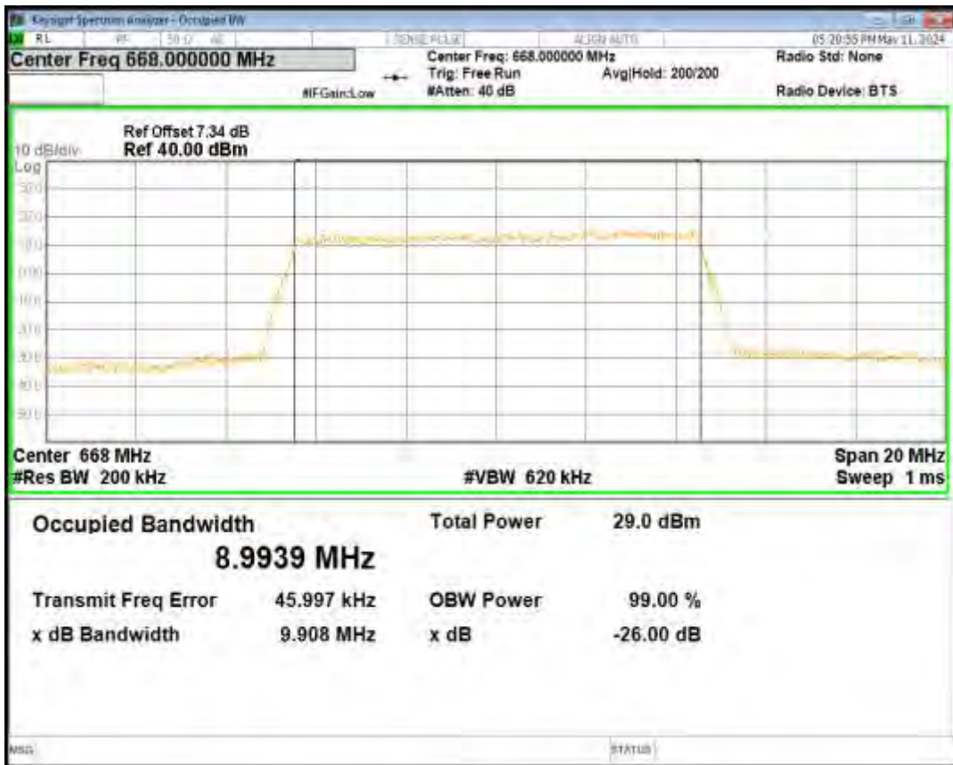
Band71 16QAM BW=10MHz Channel=133297 RB Size=50 Position=#0
