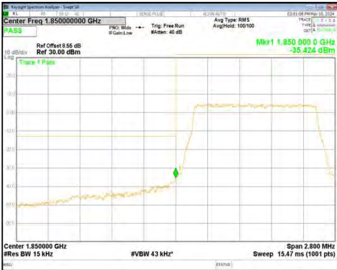
Band25 16QAM BW=5MHz Channel=26065 RB Size=25 Position=#0
