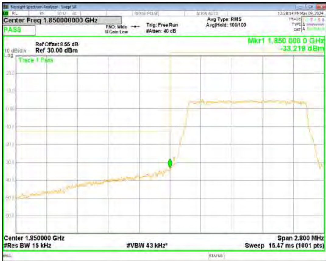
Band2 16QAM BW=1.4MHz Channel=19193 RB Size=6 Position=#0
