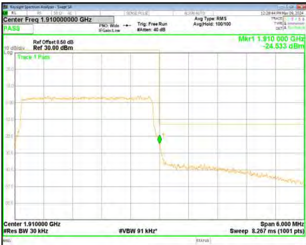
Band2 QPSK BW=10MHz Channel=18650 RB Size=50 Position=#0
