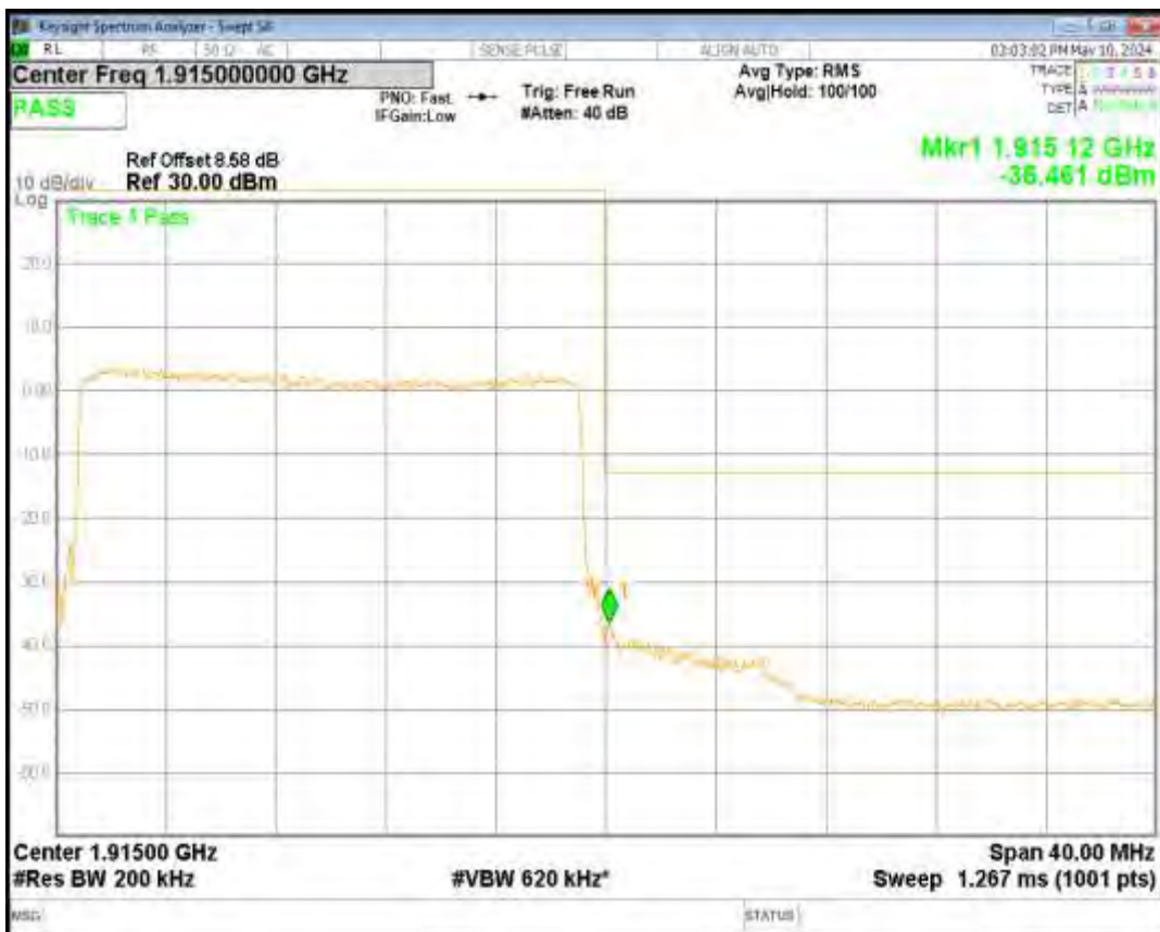
Band25 16QAM BW=3MHz Channel=26055 RB Size=15 Position=#0
