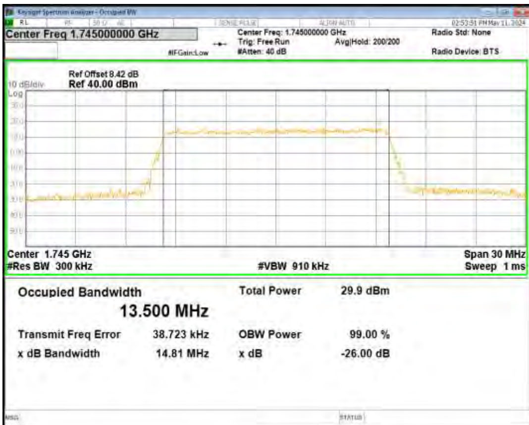
Band66 16QAM BW=15MHz Channel=132047 RB Size=75 Position=#0
