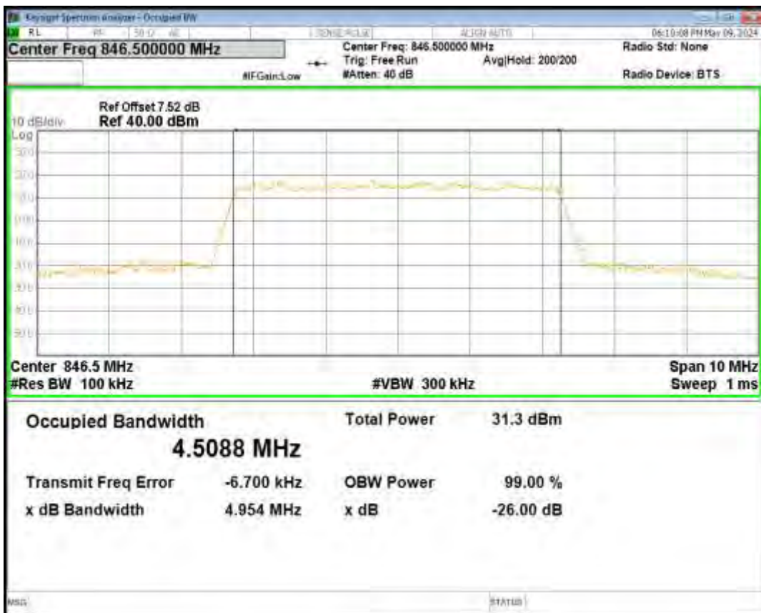
Band66 16QAM BW=1.4MHz Channel=131979 RB Size=6 Position=#0
