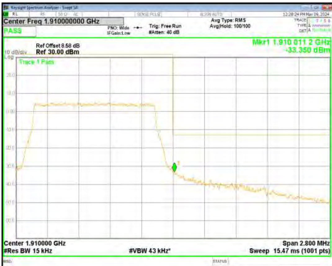
Band2 16QAM BW=10MHz Channel=18650 RB Size=50 Position=#0
