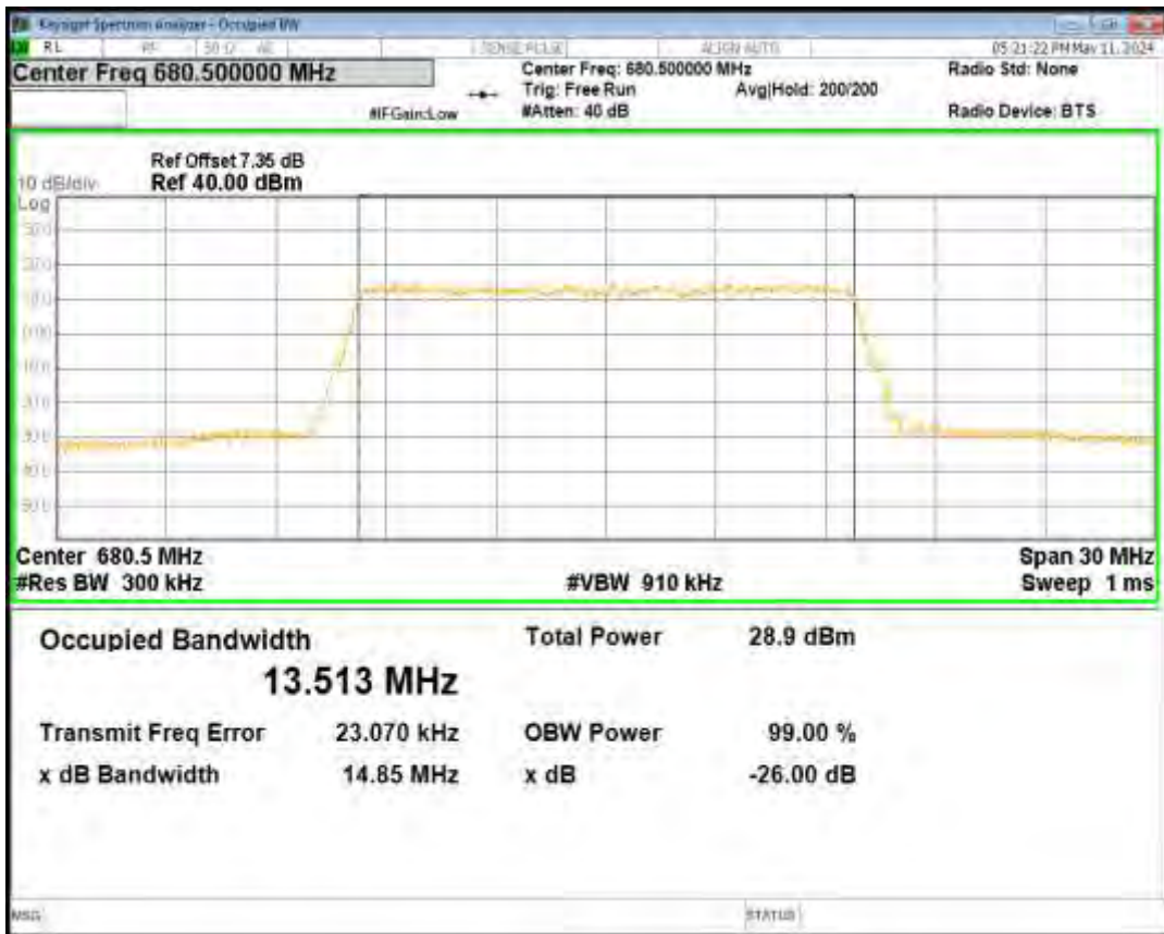
Band71 16QAM BW=15MHz Channel=133397 RB Size=75 Position=#0
