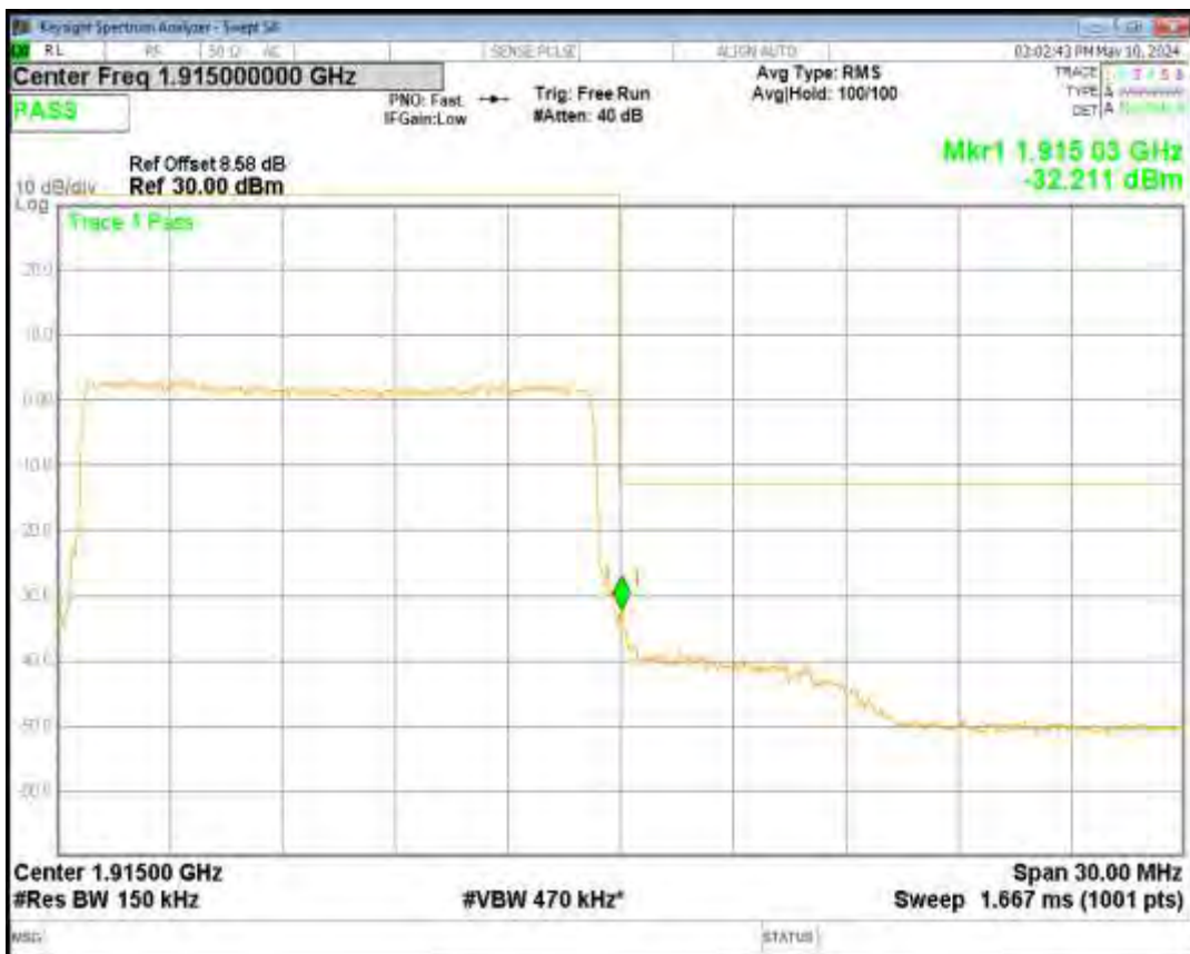
Band25 16QAM BW=20MHz Channel=26140 RB Size=100 Position=#0
