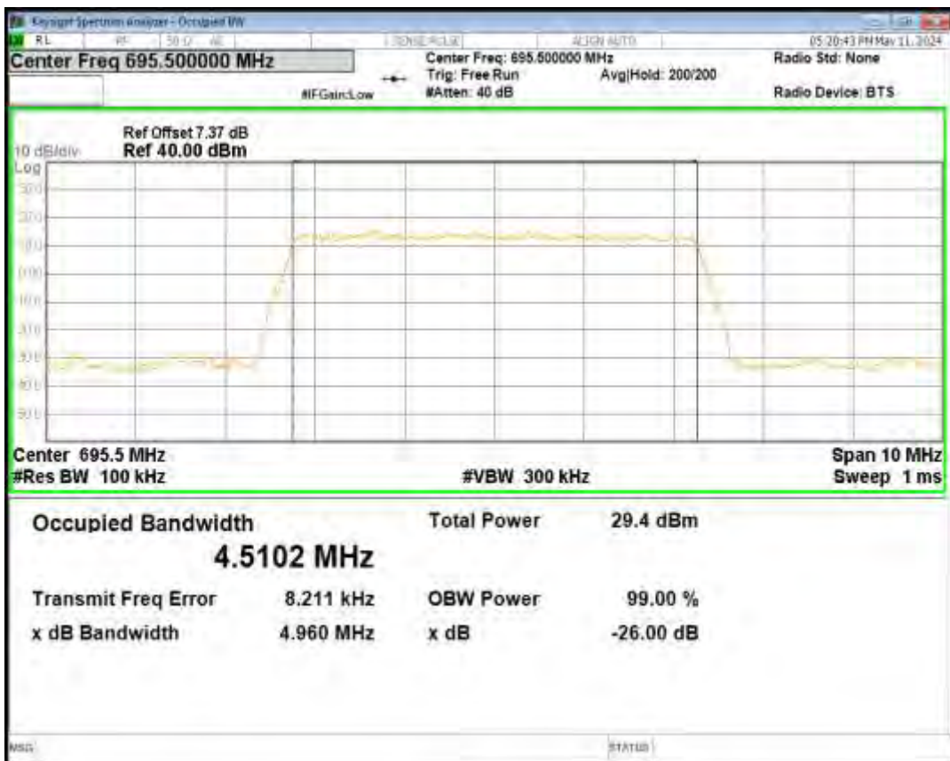
Band71 QPSK BW=5MHz Channel=133447 RB Size=25 Position=#0
