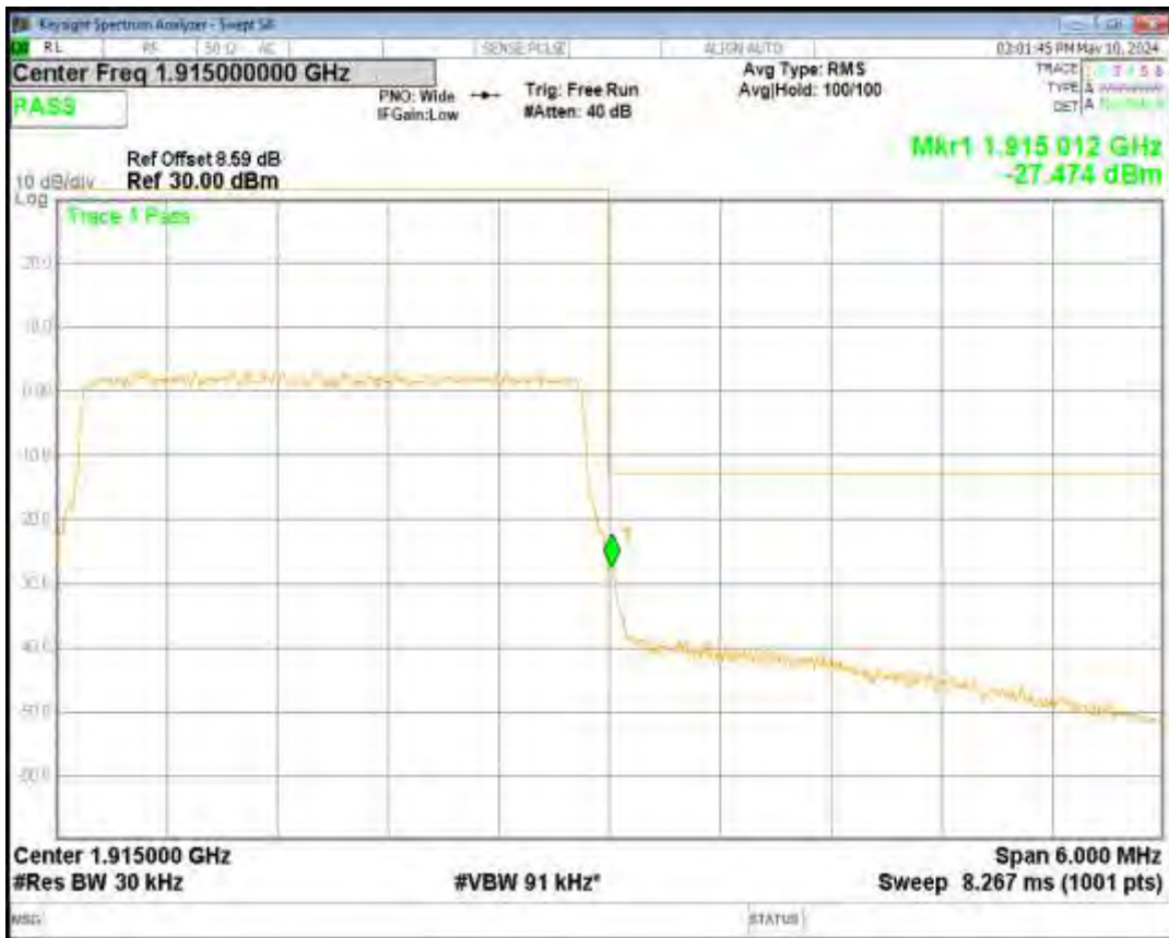
Band25 QPSK BW=10MHz Channel=26640 RB Size=50 Position=#0
