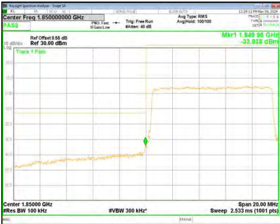
Band2 QPSK BW=10MHz Channel=19150 RB Size=50 Position=#0
