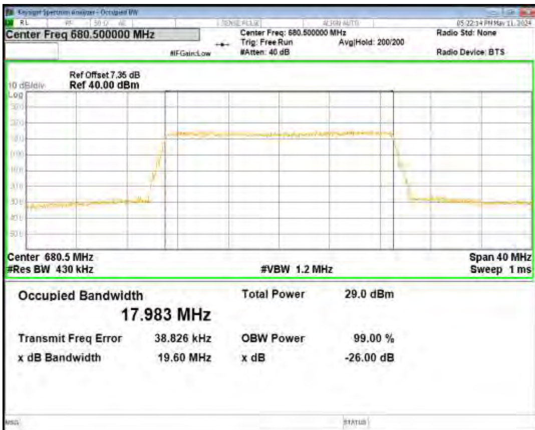
Band71 16QAM BW=20MHz Channel=133372 RB Size=100 Position=#0
