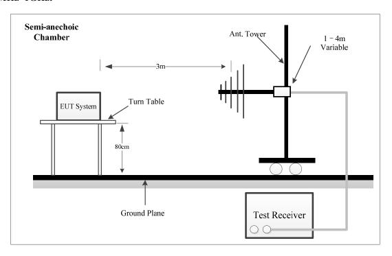
The radiated emission tests were performed in the 3-meter chamber test site, using the setup accordance with the ANSI C63.10-2020.
