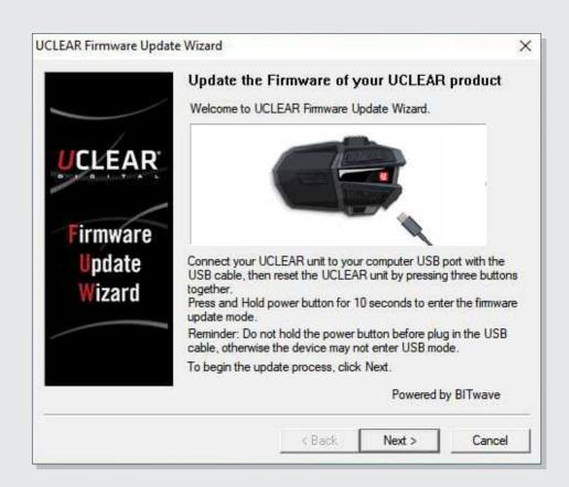
Power **OFF** state, connect device to PC/MAC with included USB charge/data cable. Hold POWER+UP+DOWN to reset device, then hold **POWER** until red LED turns off (prepares device for update).
