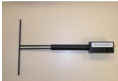
Figure 1 – Satimo COMOSAR Validation Dipole
