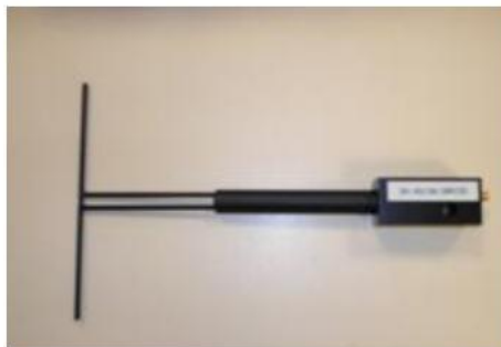
Figure 1 – Satimo COMOSAR Validation Dipole
