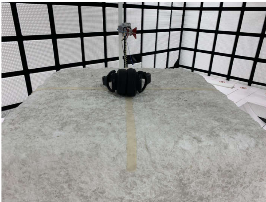
Radiated spurious emission Test Setup-2(Above 1GHz)
