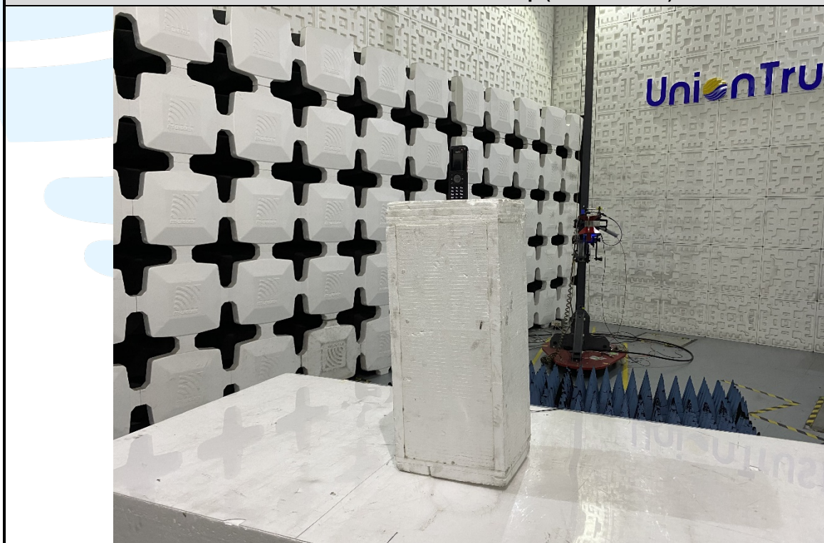
Radiated emission Test Setup (Above 1 GHz)
