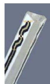
Figure 3.2 Probe Thick-Film Technique
