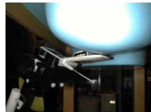
Figure 27. Left Head SAR Test Setup -- Ear / Tilt Position --
