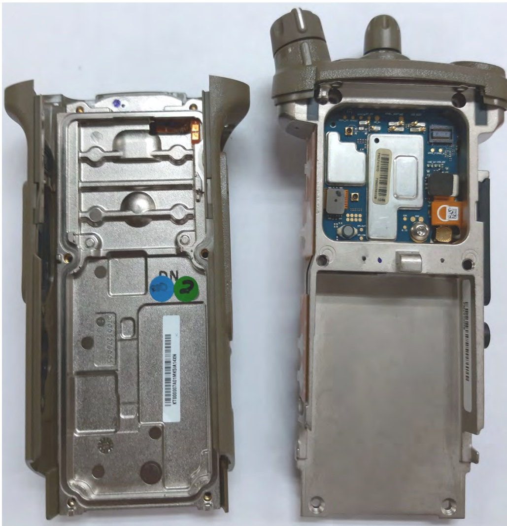
Expansion board with chassis and housing of SRX2200 Model 1.5 (Back side)
