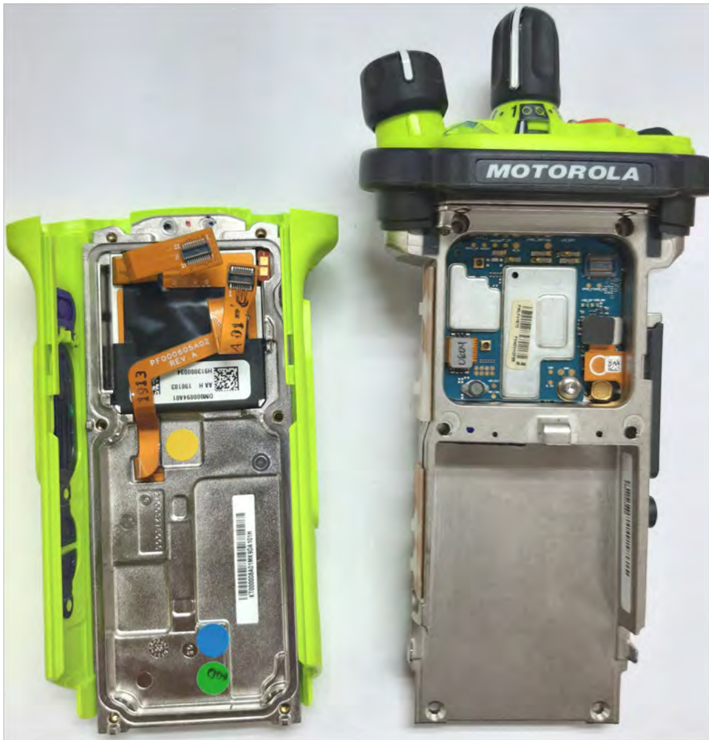
Expansion board with chassis and housing of APX6000XE Model 2.5 (Back side)
