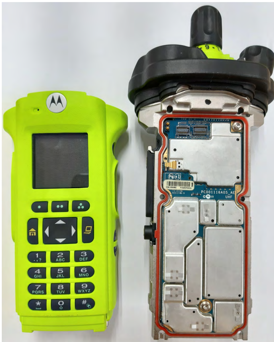
RF and Vocon boards with chassis and housing of APX6000XE Model 3.5 (Front side)
