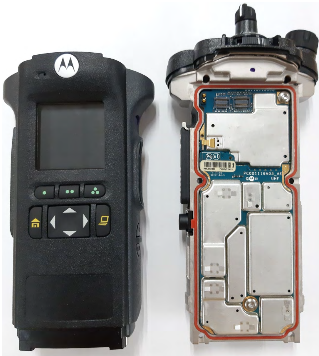
RF and Vocon boards with chassis and housing of APX6000/APX6000Li/APX5000 Model 2.5 (Front side)
