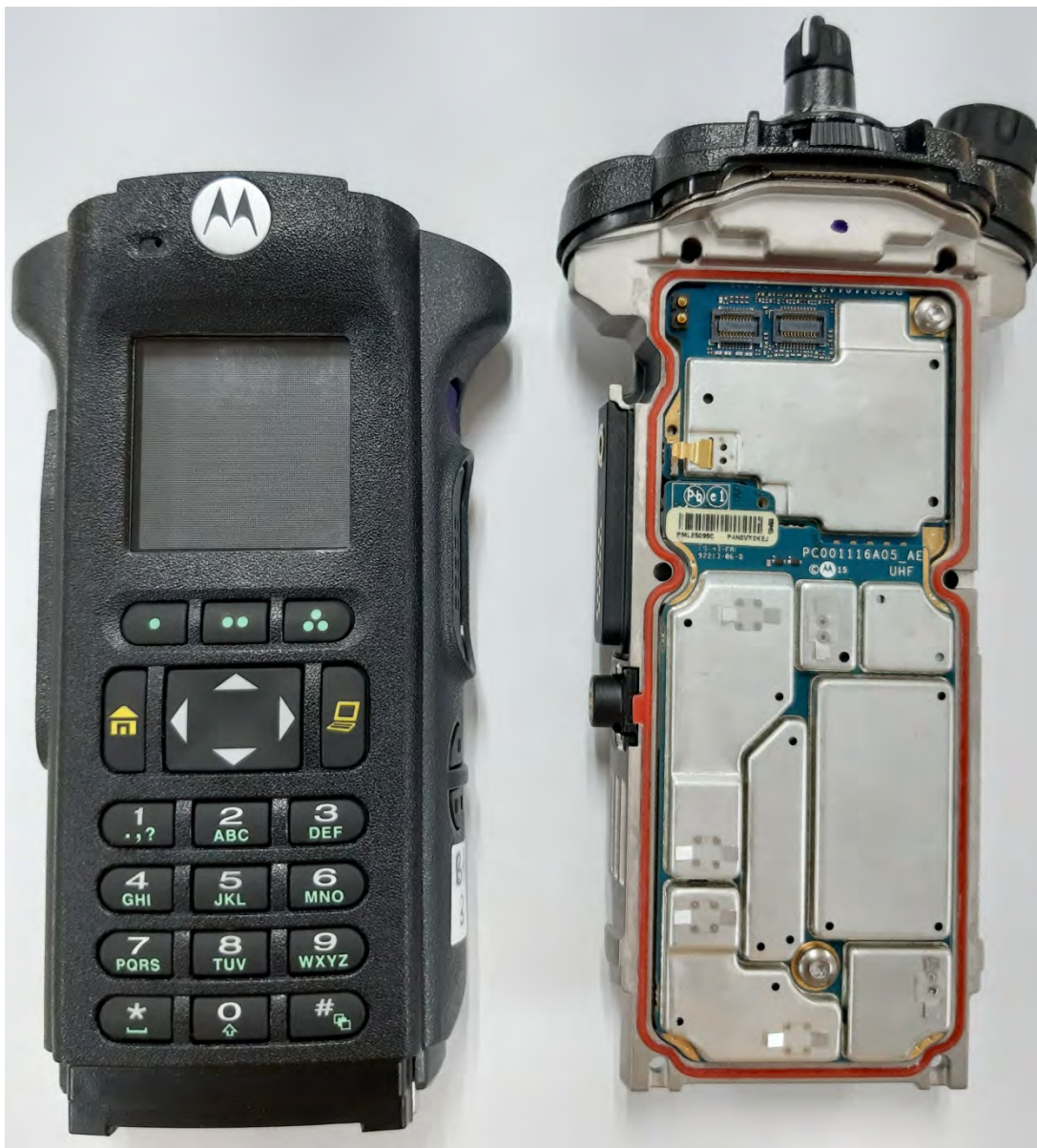
RF and Vocon boards with chassis and housing of APX6000/APX6000Li/APX5000 Model 3.5 (Front side)
