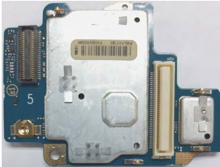
Vocon board with shields (Bottom) (APX6000/APX5000/APX6000XE/APX6000Li/SRX2200)
