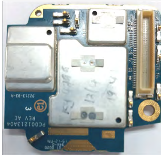
Expansion board with shields (Bottom) (APX6000/APX5000/APX6000XE/APX6000Li/SRX2200)
