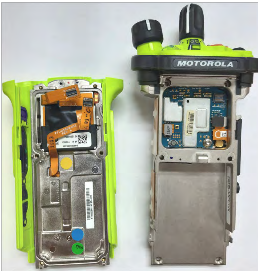
Expansion board with chassis and housing of APX6000XE Model 3.5 (Back side)
