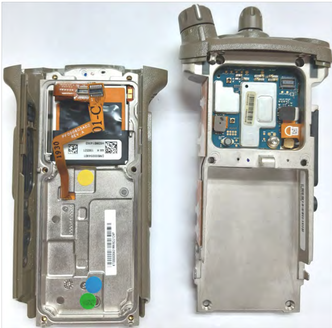
Expansion board with chassis and housing of SRX2200 Model 3.5 (Back side)
