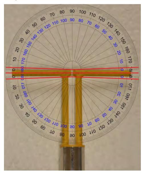
• The center red line indicates that the arms of the dipole fall within  $\pm 2^{\circ}$
