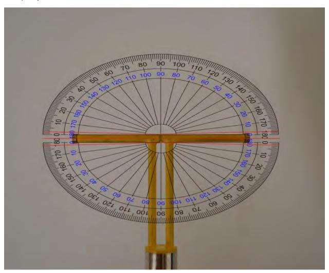
• The center red line indicates that the arms of the dipole fall within  $\pm 2^{\circ}$
