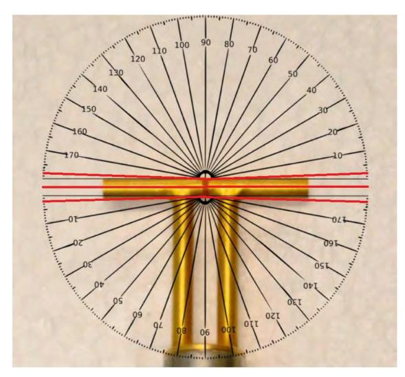
$\bullet$   $\;$  The center red line indicates that the arms of the dipole fall within  $\pm 2^{\circ}$
