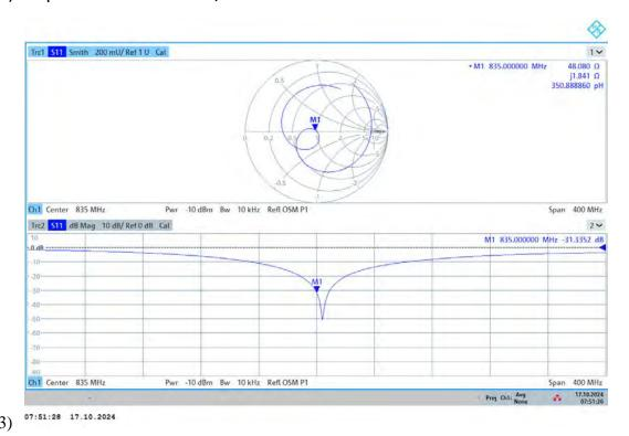
• Return/Loss is greater than the -20 dB cutoff and Impedance is within 5  $\Omega$  of previous value.
