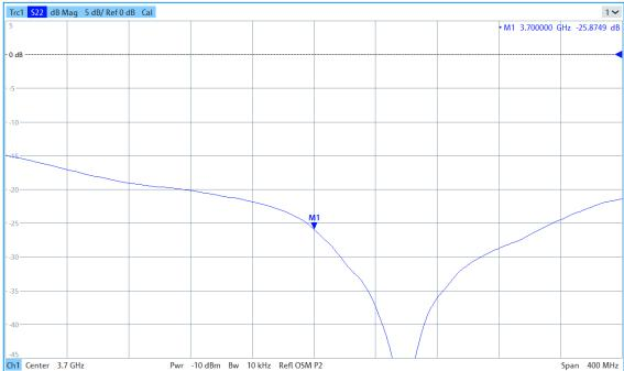
Return/Loss is greater than the -20 dB cutoff and Impedance is within 5  $\Omega$  of previous value.
