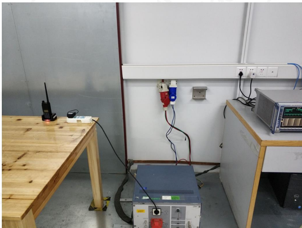
RADIATED EMISSION TEST SETUP-BELOW 1GHZ
