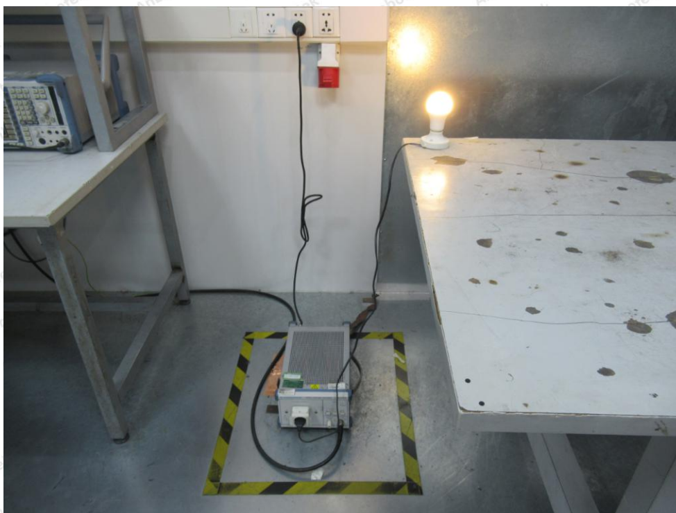
Photo of Conducted Emission Measurement
