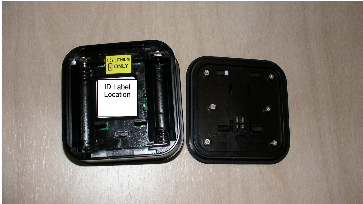
Back cover removed, Battery compartment
