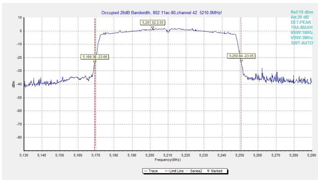
Fig. 11 Occupied 26dB Bandwidth (802. 11ac-VHT80, 5210MHz)
