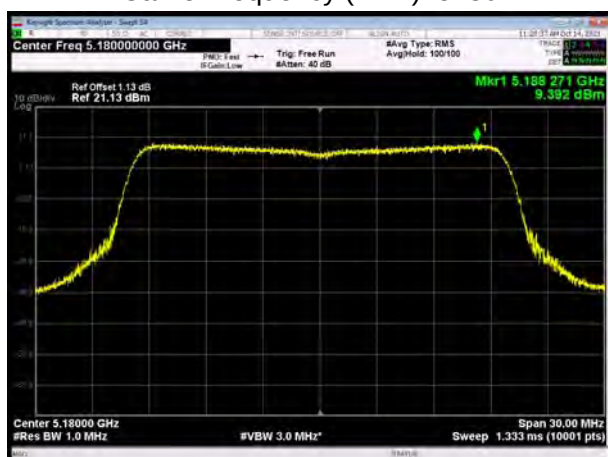
U-NII-1, 802.11ax HE20 Carrier frequency (MHz): 5200
