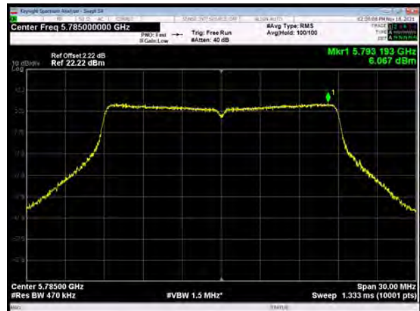
U-NII-3, 802.11n HT20 Carrier frequency (MHz): 5825
