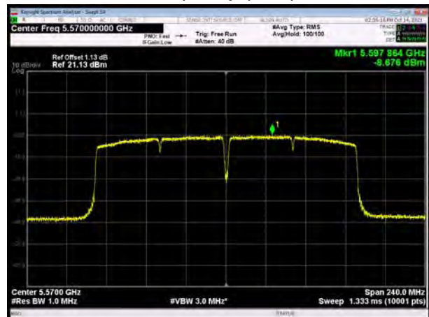
U-NII-2C, 802.11ax HE20 Carrier frequency (MHz): 5500
