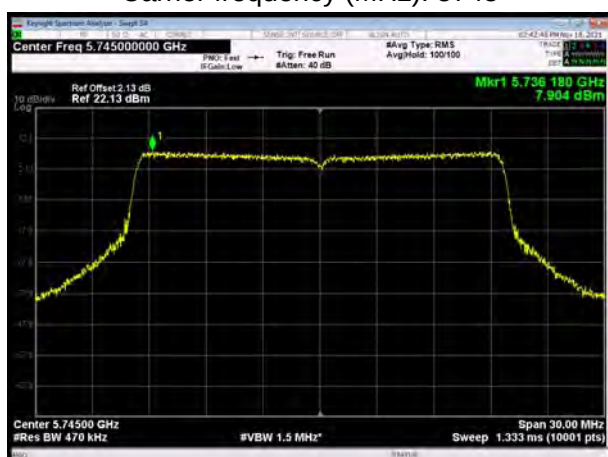
U-NII-3, 802.11ax HE20 Carrier frequency (MHz): 5745
