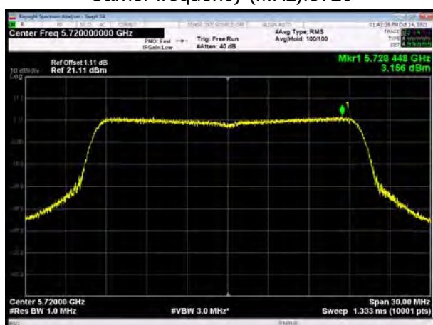
U-NII-2C, 802.11ax HE20 Carrier frequency (MHz): 5720
