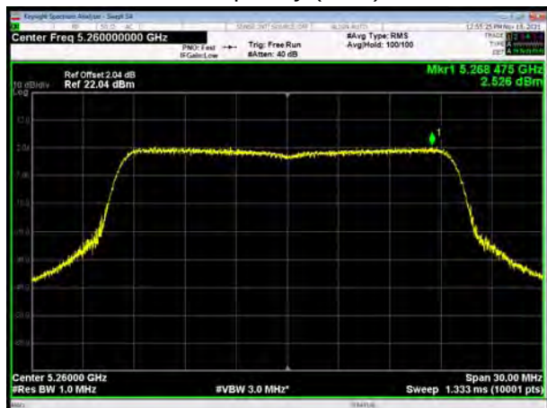
U-NII-2A, 802.11ax HE20 Carrier frequency (MHz): 5300
