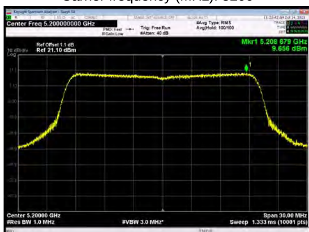
U-NII-1, 802.11ax HE20 Carrier frequency (MHz): 5200
