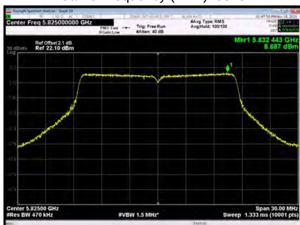
U-NII-3, 802.11n HT40 Carrier frequency (MHz): 5755
