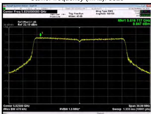
U-NII-3, 802.11ax HE20 Carrier frequency (MHz): 5825
