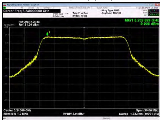
U-NII-1, 802.11a Carrier frequency (MHz): 5240
