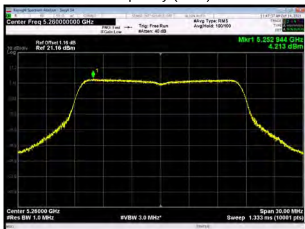
U-NII-2A, 802.11a Carrier frequency (MHz): 5300
