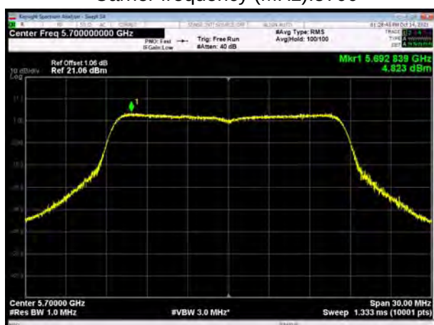
U-NII-2C, 802.11a Carrier frequency (MHz):5700
