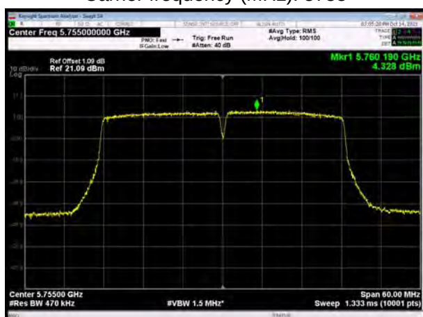
U-NII-3, 802.11n HT40 Carrier frequency (MHz): 5755
