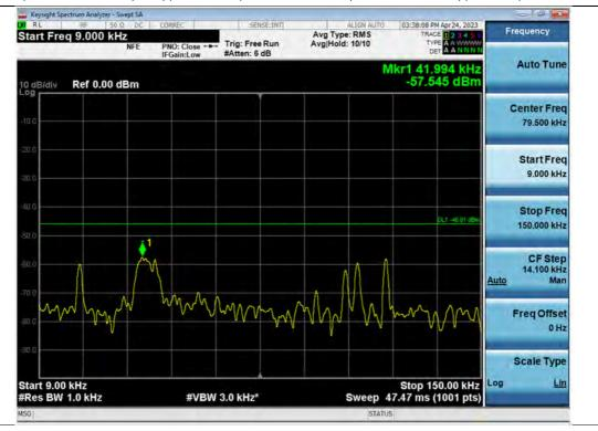
Spurious / 3.7 GHz Service (Ant2) / Downlink / 5G NR 4 Carriers(100 + 60 + 80 + 40) / Middle / 9 kHz ~ 150 kHz
