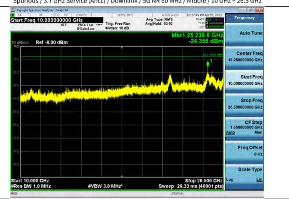
Spurious / 3.7 GHz Service (Ant1) / Downlink / 5G NR 60 MHz / Middle / 10 GHz ~ 26.5 GHz
