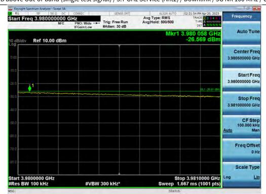
+3 dB above Out-of-band (single test signal) / 3.7 GHz Service (Ant2) / Downlink / 5G NR 100 MHz / Upper
