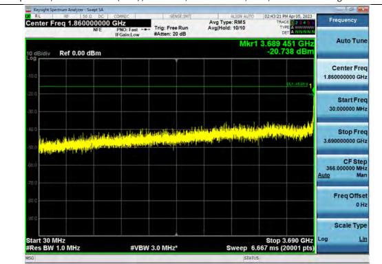
Spurious / 3.7 GHz Service (Ant1) / Downlink / 5G NR 80 MHz / Low / 30 MHz ~ Low Edge - 10 MHz
