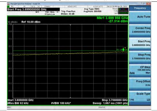
+3 dB above Out-of-band (single test signal) / 3.7 GHz Service (Ant2) / Downlink / 5G NR 60 MHz / Lower
