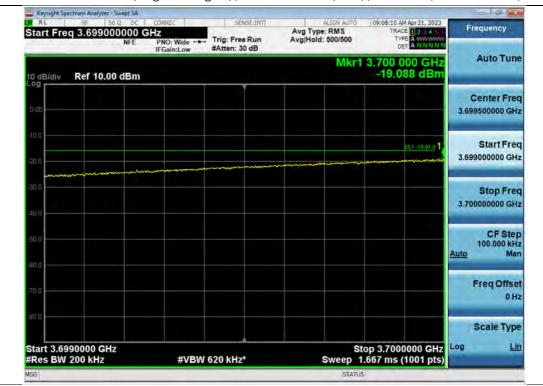
+3 dB above Out-of-band (single test signal) / 3.7 GHz Service (Ant2) / Downlink / 5G NR 20 MHz / Lower
