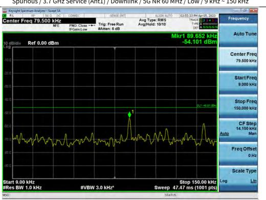
Spurious / 3.7 GHz Service (Ant1) / Downlink / 5G NR 60 MHz / Low / 9 kHz ~ 150 kHz
