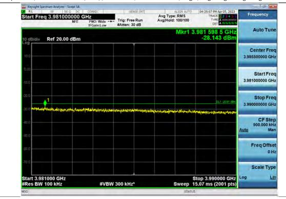
Spurious / 3.7 GHz Service (Ant1) / Downlink / 5G NR 40 MHz / High / High Edge ~ High Edge + 10 MHz
