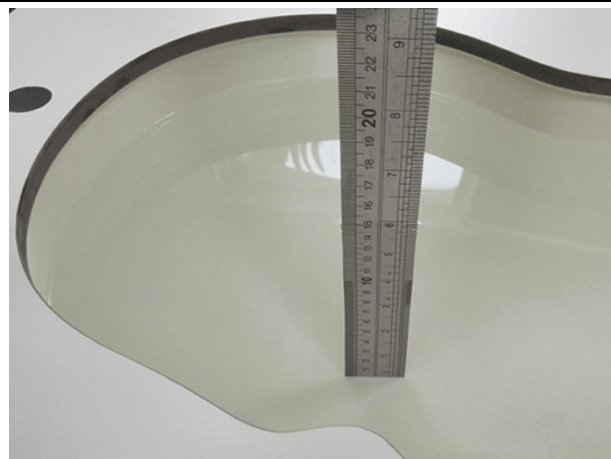
Liquid depth in the head phantom (2450MHz)
