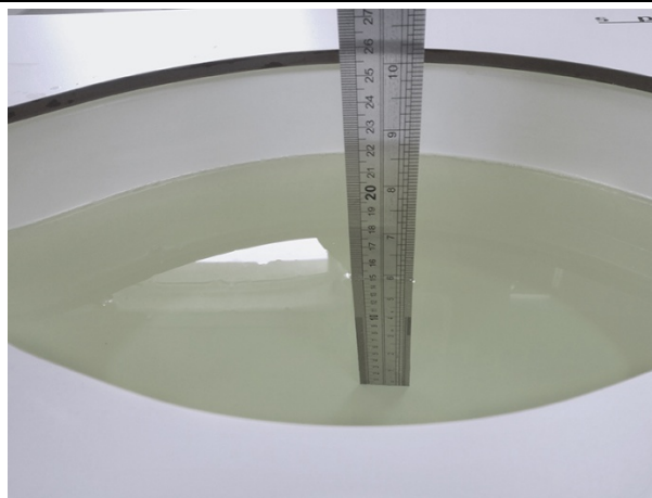
Liquid depth in the body phantom (2450MHz)
