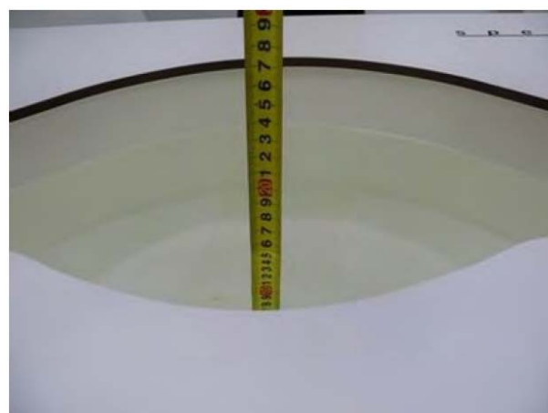
Liquid depth in the body phantom (1900MHz)
