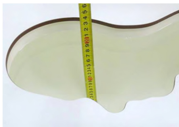
Liquid depth in the head phantom (835MHz)
