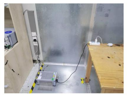
Radiated Emissions From 30MHz-1000MHz
