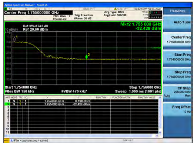
Band4 / 15MHz / High CH / QPSK / FULL RB
