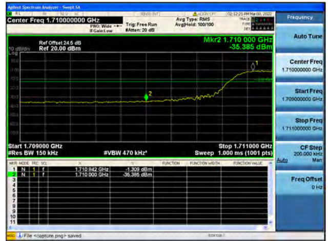
Band4 / 15MHz / High CH / QPSK / FULL RB
