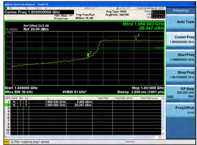
Band25 / 1.4MHz / High CH / QPSK / FULL RB
