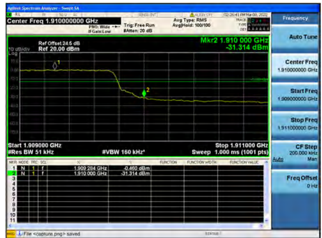
Band2 / 5MHz / High CH / QPSK / FULL RB
