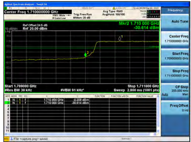
Band4 / 3MHz / High CH / QPSK / FULL RB
