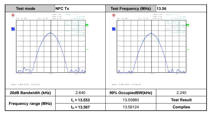
C.1 Test Result of 20dB Spectrum Bandwidth
