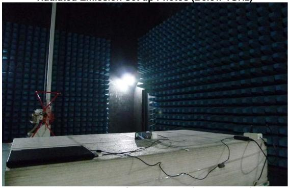
Radiated Emission Set up Photos (Above 1GHz)
