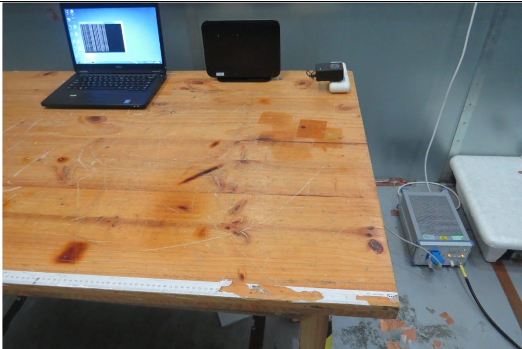
Picture 3 Conducted Emission Test Setup
