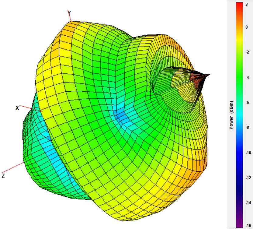
Figure 4-4. 2.4GHz Antenna 3D. 2442MHz
