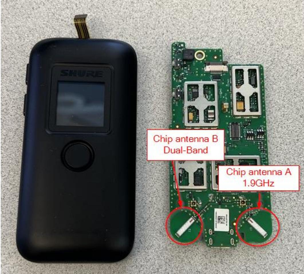
Figure 1-1. Shure MXW1X Internal Antennas Overview
