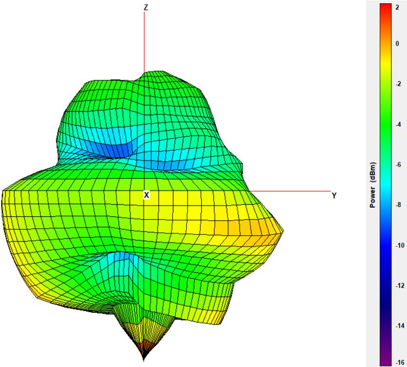
Figure 4-2. 2.4GHz Antenna Y-Z plane. 2442MHz
