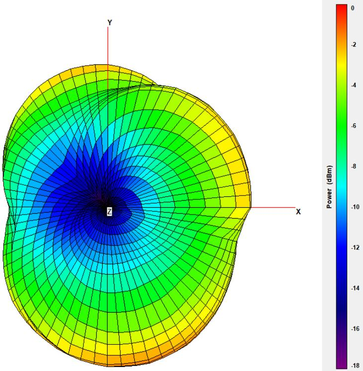
Figure 3-1. 1.9GHz Antenna B X-Y Plane.
