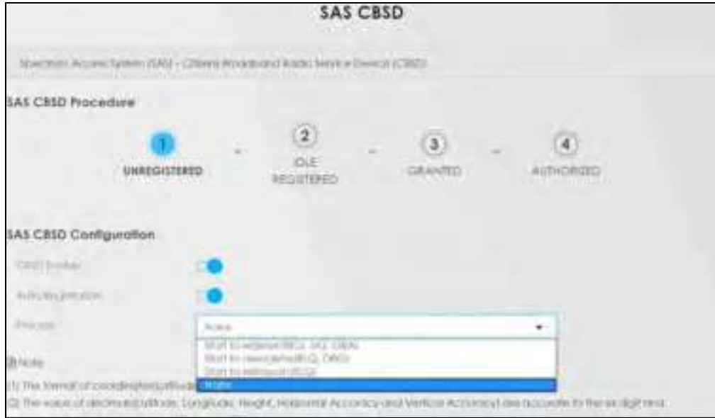
Figure 140 Network Setting > SAS CBSD > Unregistered
