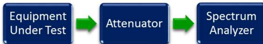
Figure 3: Spurious Emission at Antenna Terminal Test setup
