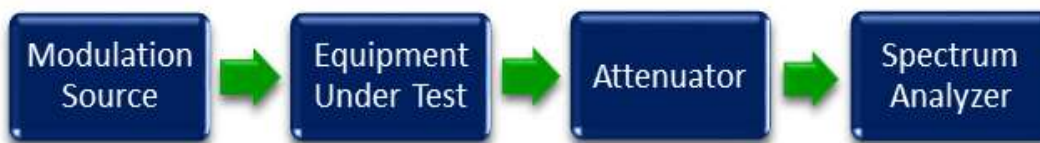
Figure 2: Occupied Bandwidth Test Setup
