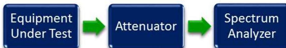
Figure 1 Output RF power Test Setup
