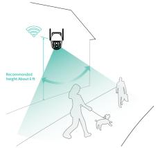
• For outdoor use, please install the camera upside down to maximize the waterproof performance and the human body infrared sensor's effectivity.
