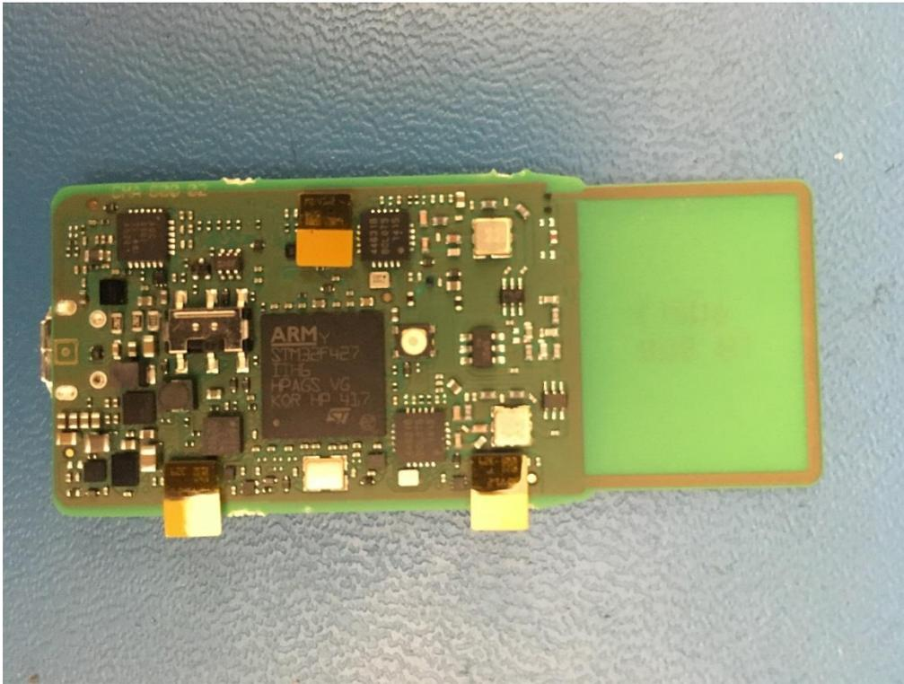
PC board front with antenna at right
