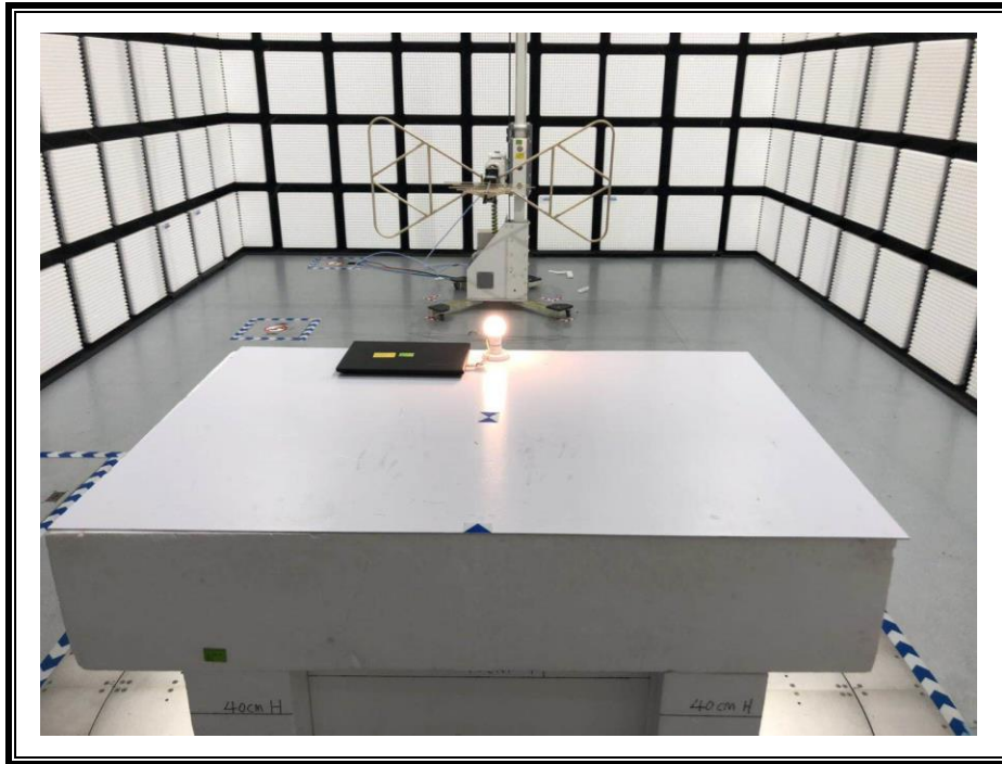
RADIATED RF MEASUREMENT SETUP (Below 30MHz)
