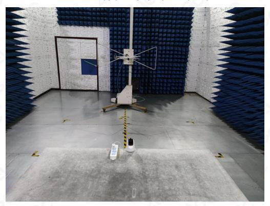
RADIATED EMISSION TEST SETUP ABOVE 1GHz
