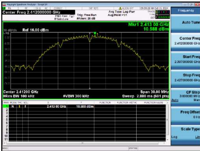
802.11b LOW CHANNEL, CARRIER LEVEL
