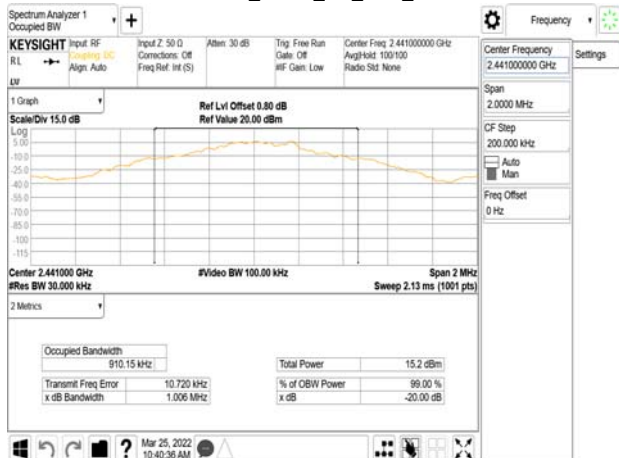
IC OBW 99%_GFSK_1M_DH5_2480MHz
