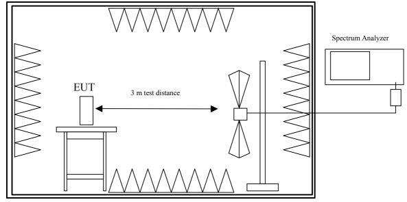
Fully anechoic chamber
