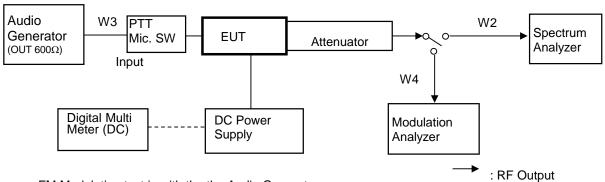
FM Modulation test is with the the Audio Generator.
